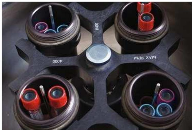
**FIGURE 1.12** Properly loaded centrifuge.
