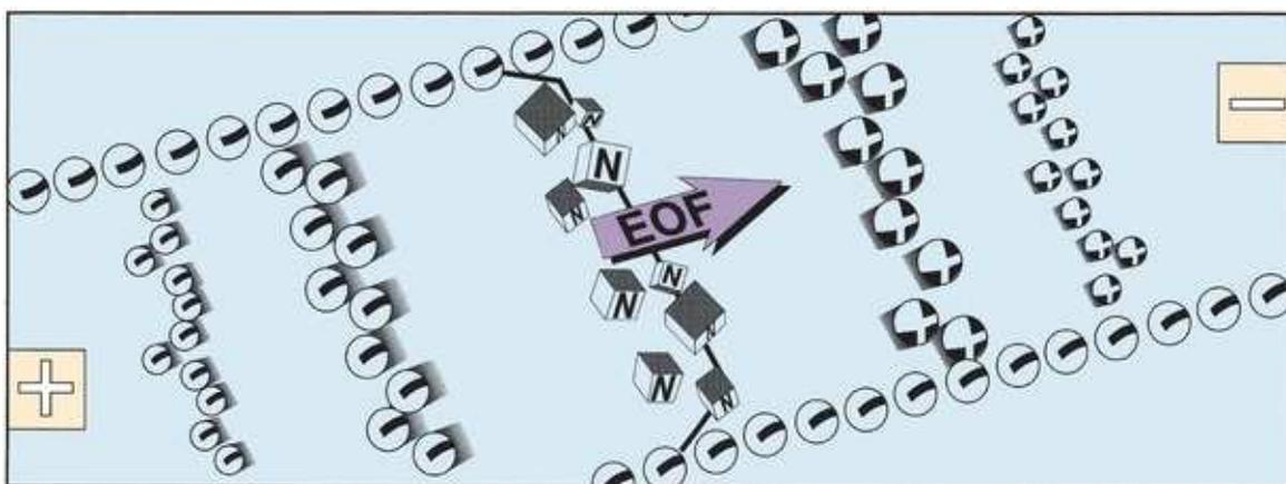
**FIGURE 5.25** Differential solute migration superimposed on electro-osmotic flow in capillary zone electrophoresis. (Adapted from Heiger DN. High-Performance Capillary Electrophoresis. Waldbronn, Germany: Hewlett-Packard; 1992.)
