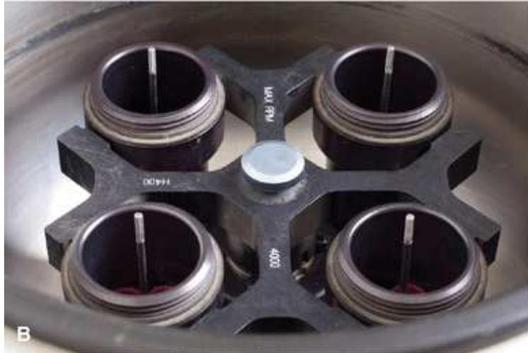
**FIGURE 1.10 (A)** Benchtop centrifuge. **(B)** Swinging-bucket rotor.
