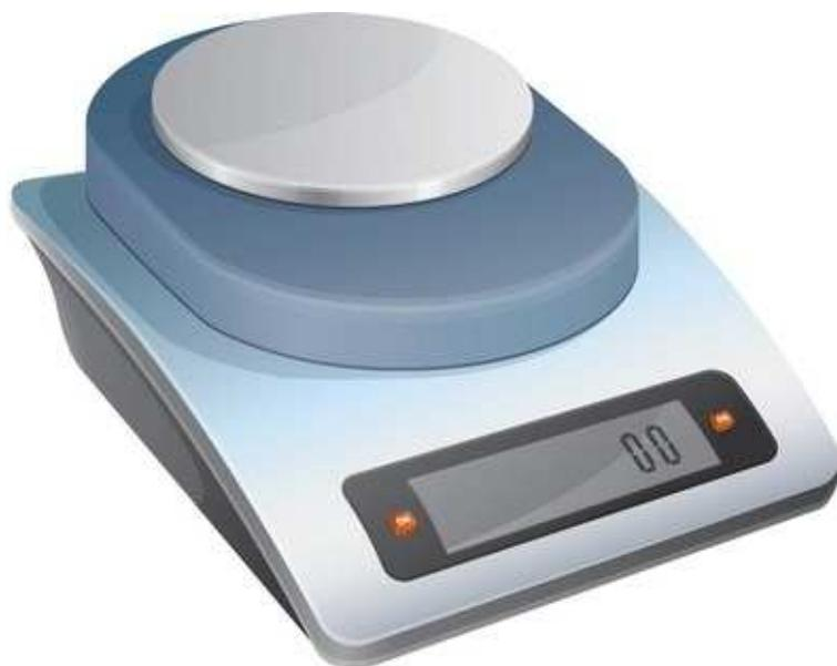
**FIGURE 1.9** Electronic top-loading balance.
