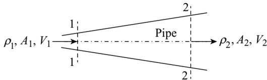
Figure 6.5 Fluid flow through a pipe
