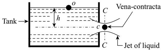
**Figure 10.1** A circular sharp-edged orifice discharging free
