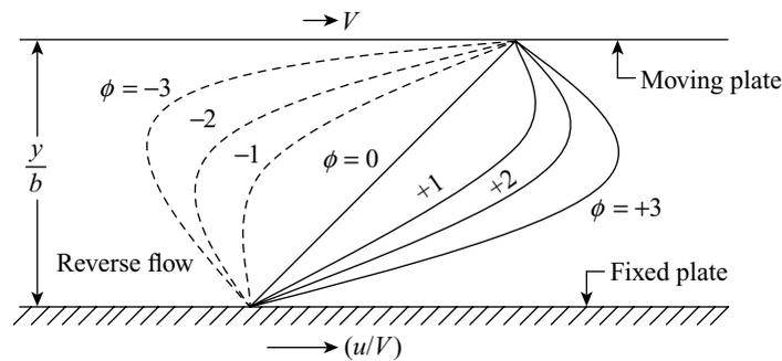
**Figure 12.13** Non-dimensional velocity curves for Couette flow
