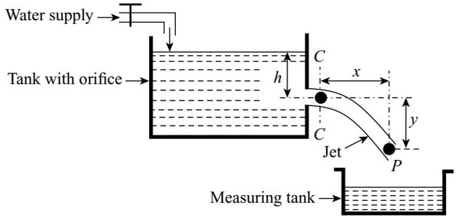
Figure 10.2 Determination of hydraulic coefficients
