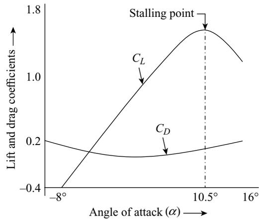
**Figure 16.10** Variation of lift and drag coefficients with angle of attack
