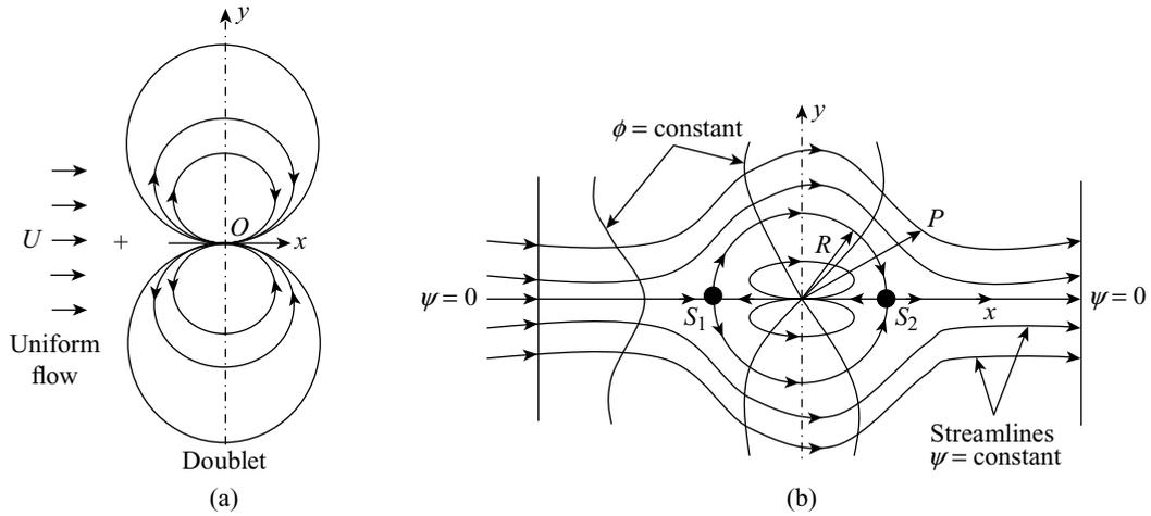
**Figure 9.19** Doublet in a uniform flow
