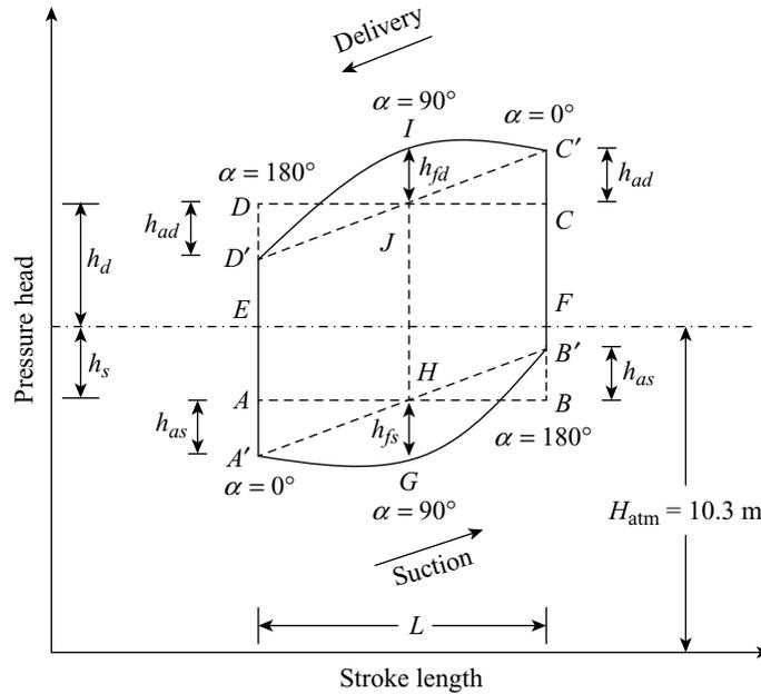
**Figure 26.9** Effect of acceleration and friction on indicator diagram
