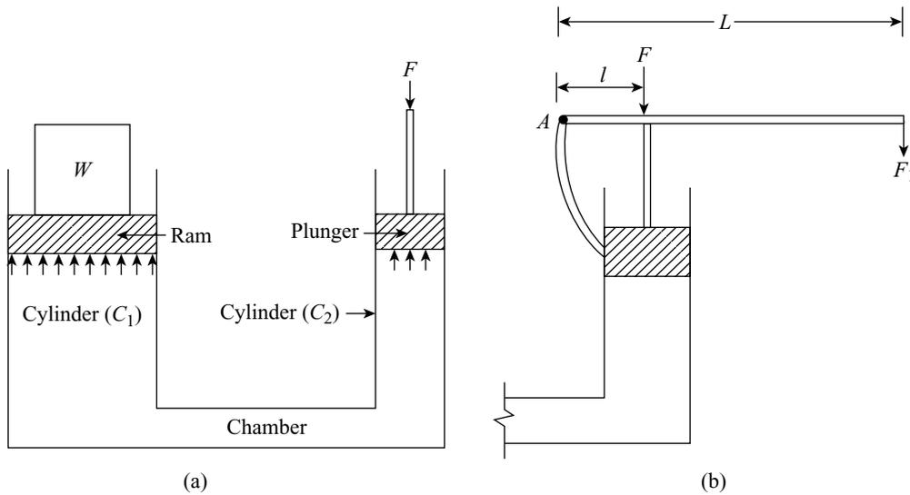
**Figure 27.1** Working of a hydraulic press
