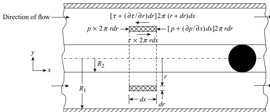
Figure 12.9 Laminar flow through an annulus
