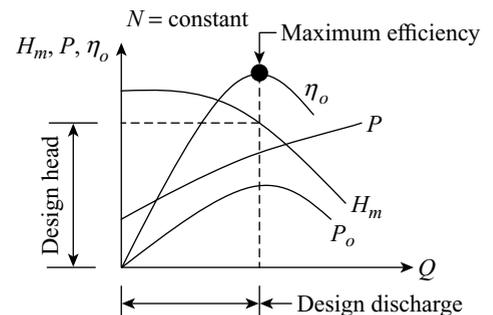
Figure 25.20 Operating characteristic curves
