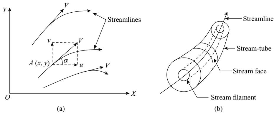
**Figure 6.1** Streamlines and stream-tube
