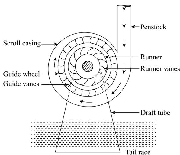
Figure 22.2 Radial flow reaction turbine
