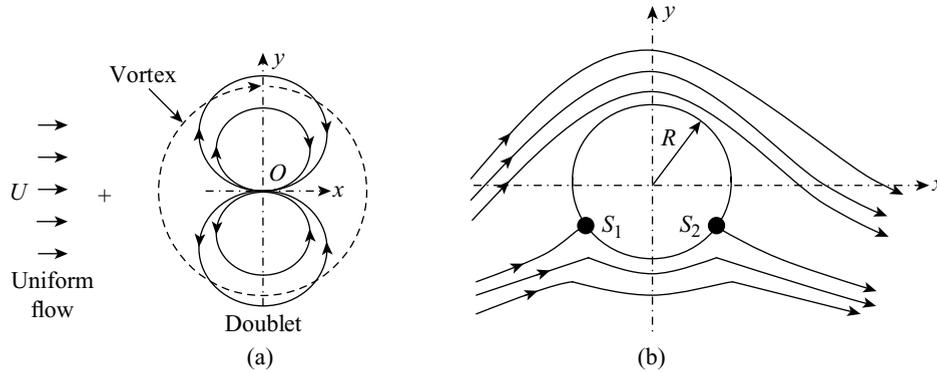
**Figure 9.24** Flow past a cylinder with circulation
