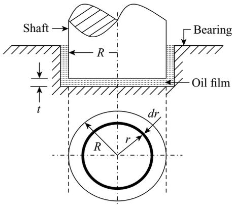
**Figure 12.16** Foot step bearing
