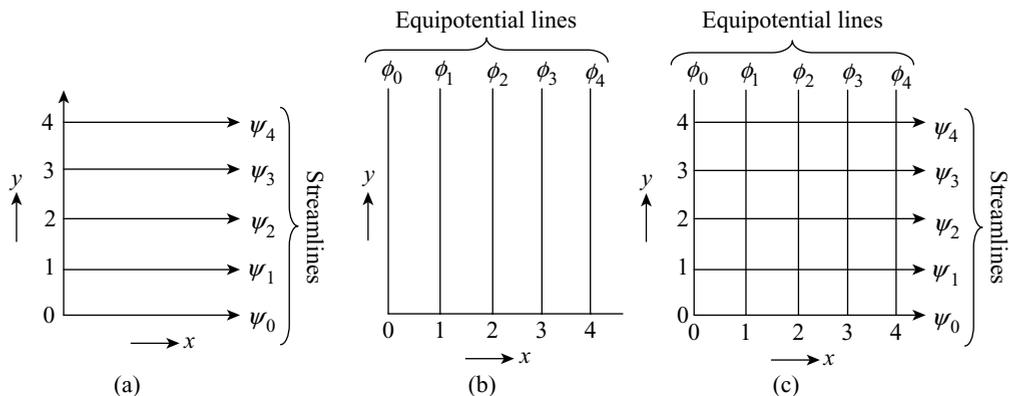
**Figure 9.2** Uniform flow parallel to  $x$ -axis
