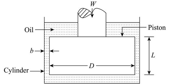
Figure 12.18 A dashpot mechanism
