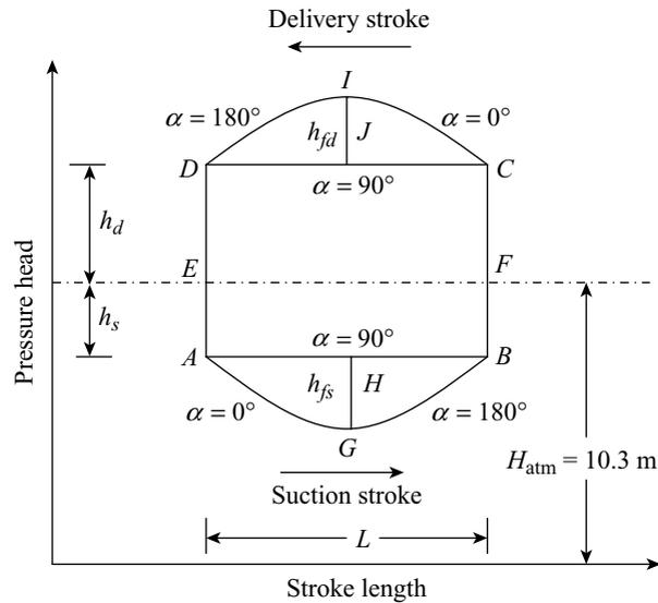
**Figure 26.8** Effect of friction on indicator diagram
