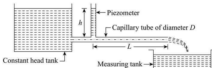
**Figure 12.19** Capillary tube viscometer
