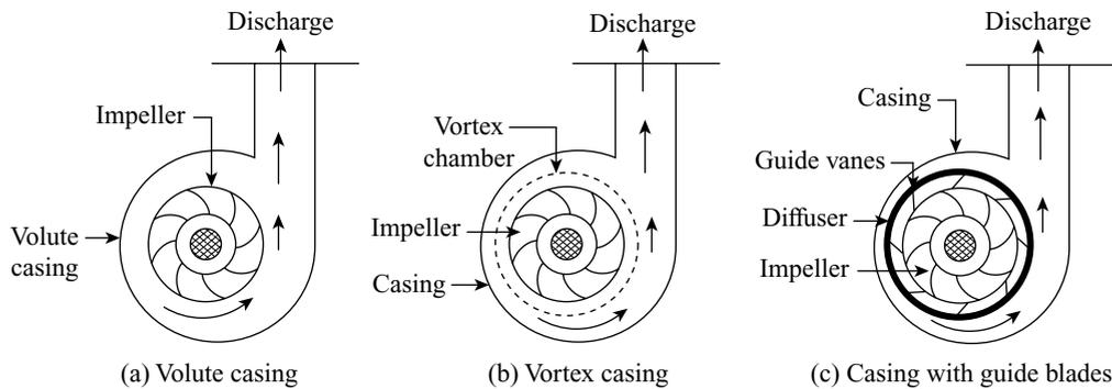
**Figure 25.5** Types of casing
