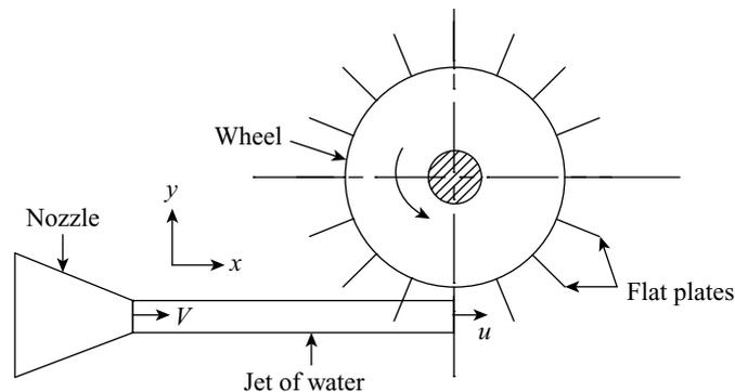
Figure 20.6 Jet striking a series of flat plates
