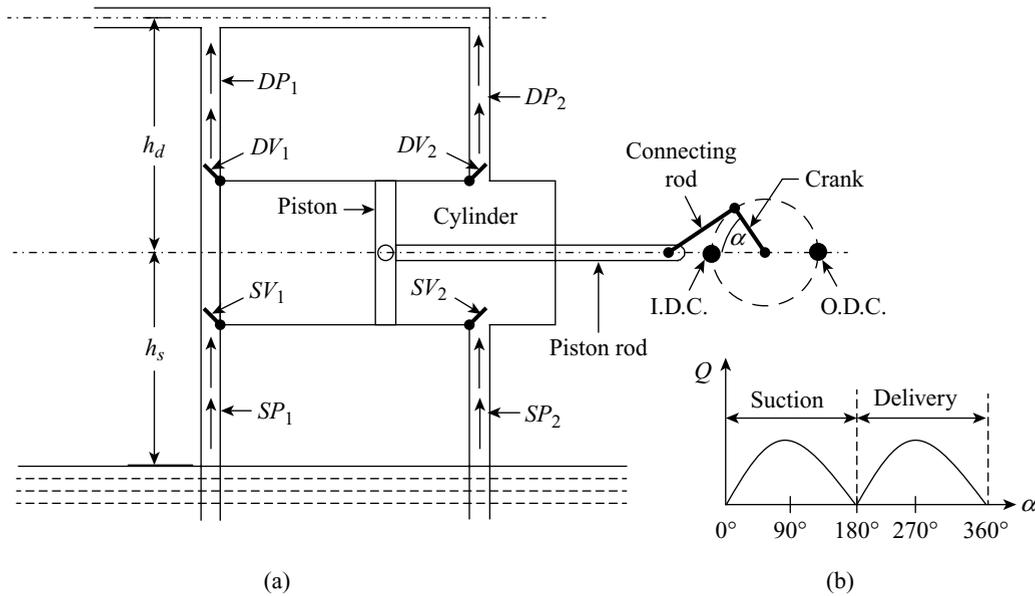
Figure 26.3 (a) Double acting reciprocating pump (b) Variation of discharge
