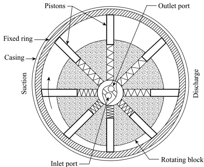
**Figure 26.18** *Radial piston pump*
