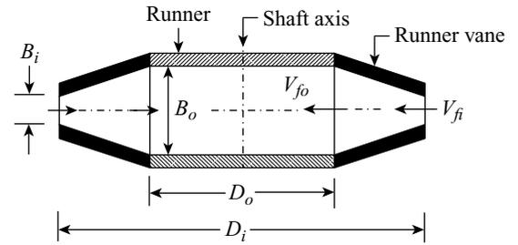
Figure 22.9 Flow entry to runner vane
