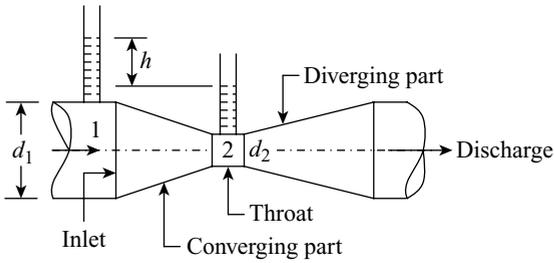
**Figure 17.6** Horizontal venturimeter carrying compressible fluid
