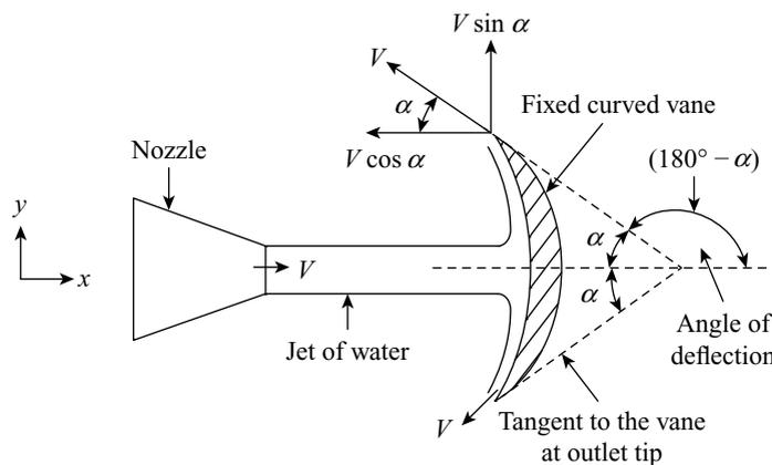
Figure 20.7 Jet striking a fixed symmetrical curved vane at its centre
