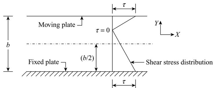
**Figure 12.14** Shear stress distribution for Couette flow
