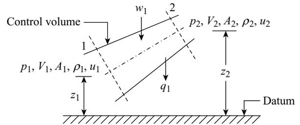
**Figure 7.2** Bernoulli's equation from energy equation
