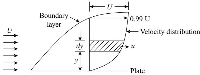
**Figure 15.2** Displacement thickness
