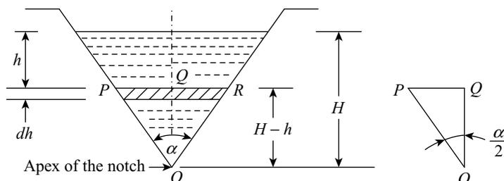
**Figure 11.5** Discharge from a triangular notch or weir
