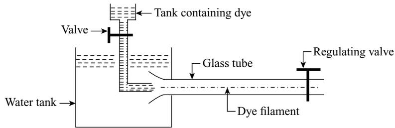
**Figure 12.1** Schematics of Reynolds experimental set-up
