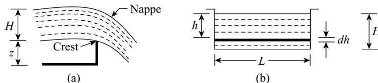
Figure 11.2 Discharge from a rectangular notch or weir
