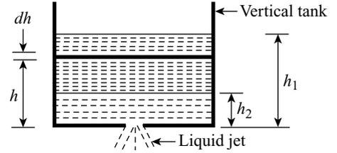
Figure 10.10 Vertical tank with an orifice at its bottom
