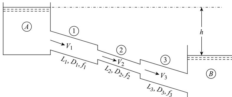
Figure 14.13 Pipes in series (compound pipes)
