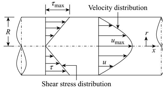
**Figure 12.6** Shear stress and velocity distribution for laminar flow in a pipe
