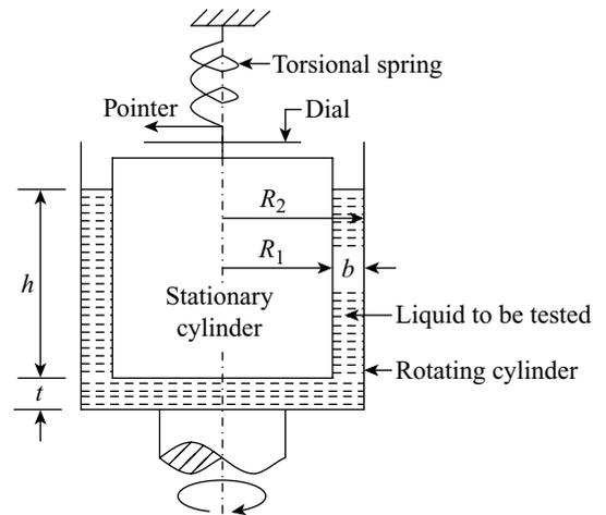
Figure 12.20 Rotating cylinder viscometer
