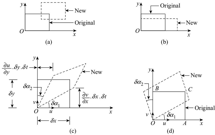
Figure 6.10 Displacement of fluid particles
