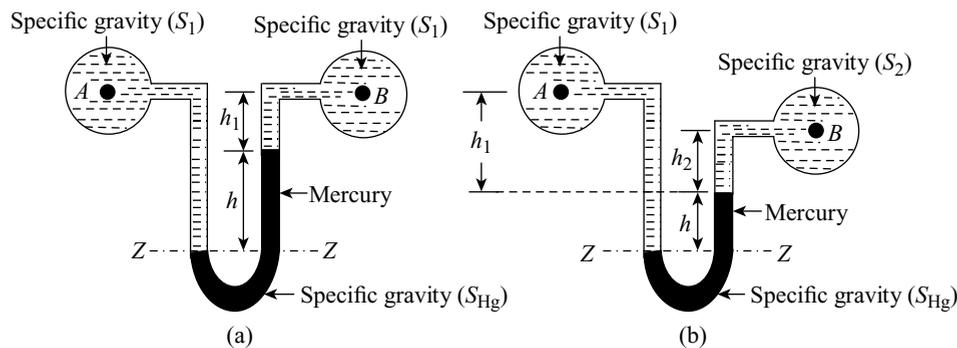
Figure 2.20 U-tube differential manometers
