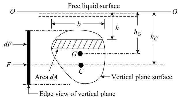
**Figure 3.3** Vertical submerged plane surface
