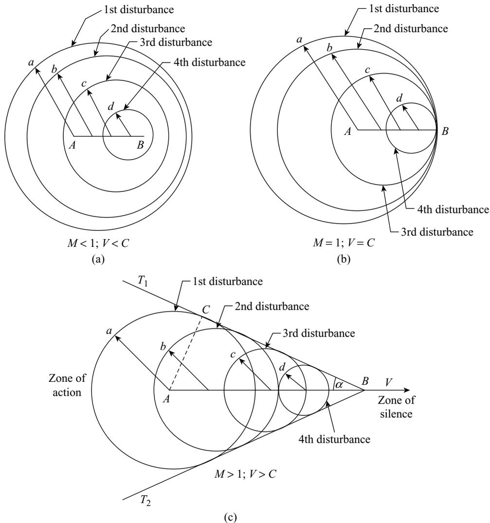
**Figure 17.2** Pressure wave propagation in a compressible fluid
