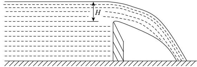
Figure 11.11 Narrow or sharp-crested weir
