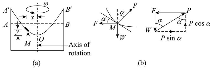
**Figure 4.8** Liquid container subjected to constant rotation
