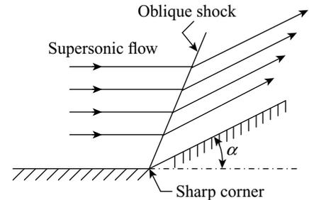
**Figure 17.8** Oblique shock wave over a concave corner
