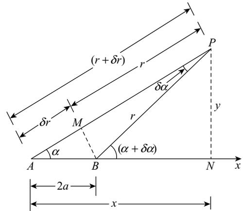
Figure 9.17 Analysis of a doublet
