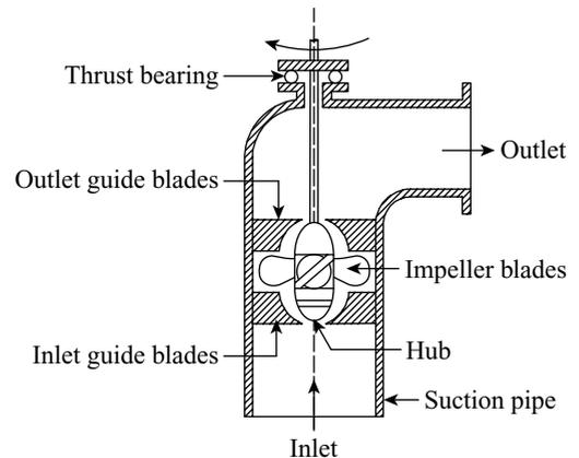
Figure 25.24 Axial flow pump
