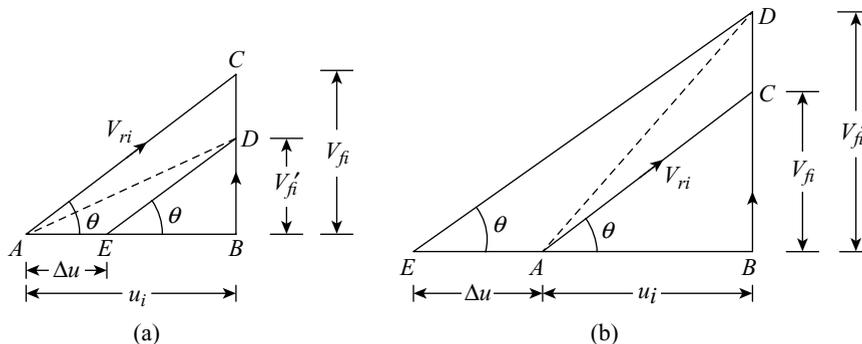
Figure 25.9 Inlet velocity triangles with decreased and increased flow
