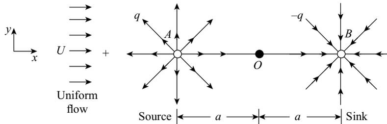
**Figure 9.21** Superposition of uniform flow over source-sink pair
