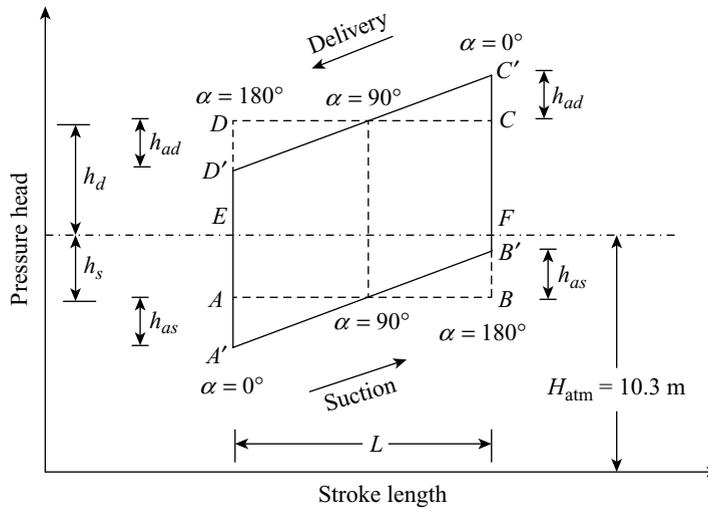
**Figure 26.6** Effect of acceleration on indicator diagram
