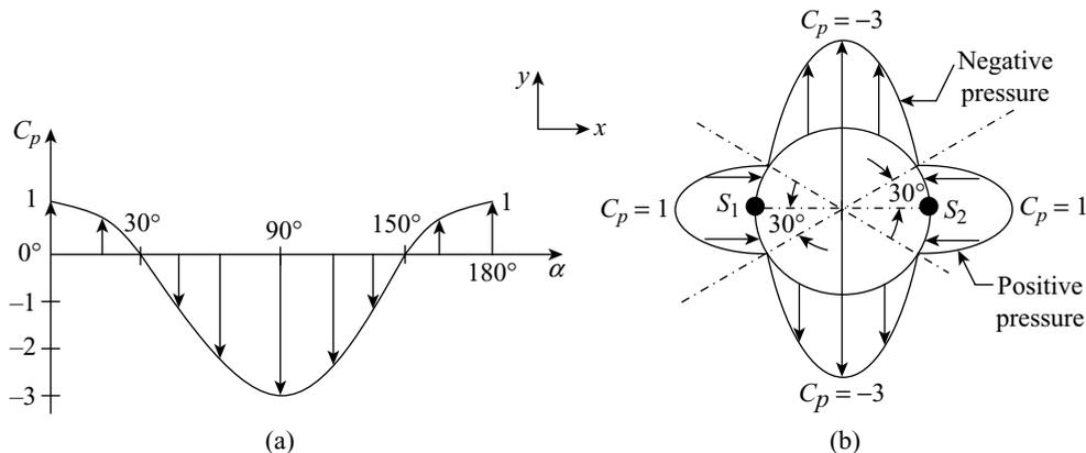
**Figure 9.20** Pressure distribution over the surface of a cylinder
