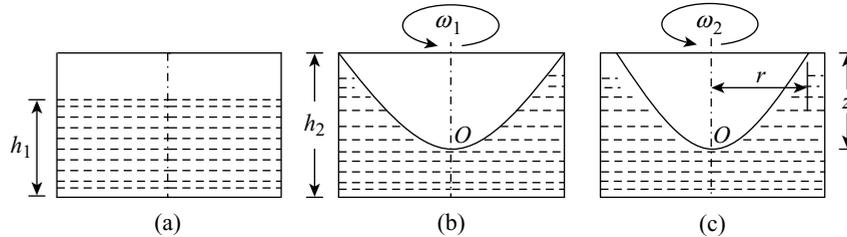
Figure 8.8 Rotation of liquid in a closed cylinder
