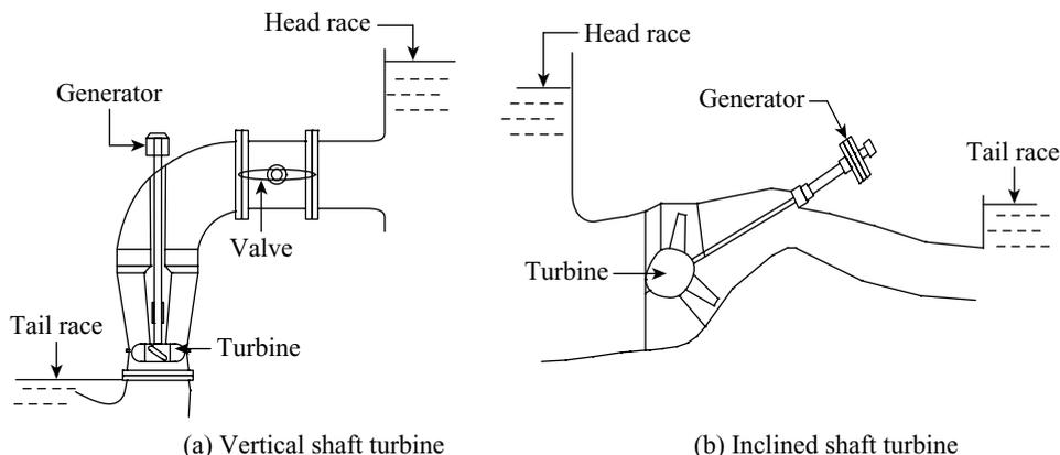
**Figure 23.10** Tubular turbine
