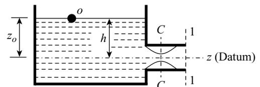
Figure 10.14 External cylindrical mouthpiece
