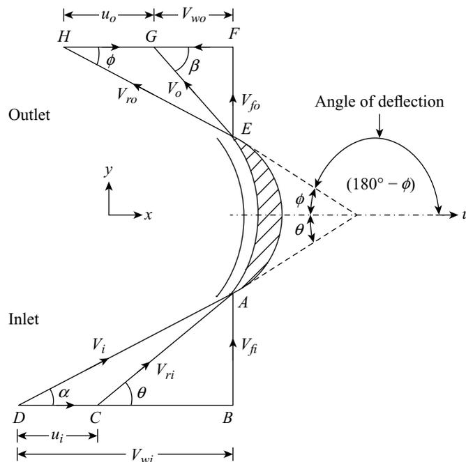
Figure 20.11 Jet strikes tangentially at the tip of moving unsymmetrical curved vane
