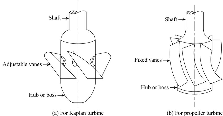
**Figure 23.1** Runners of Kaplan and propeller turbines
