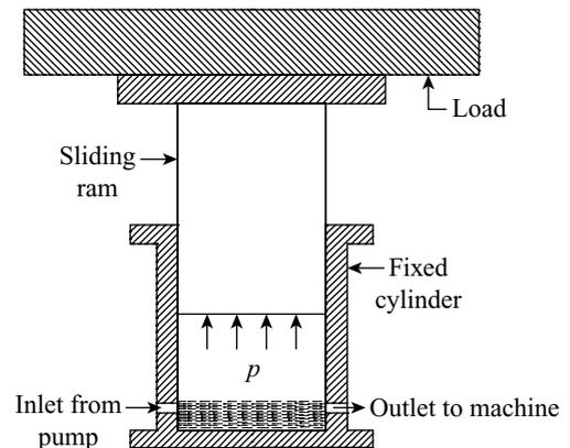
**Figure 27.3** Simple hydraulic accumulator
