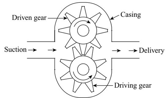
Figure 27.15 External gear pump
