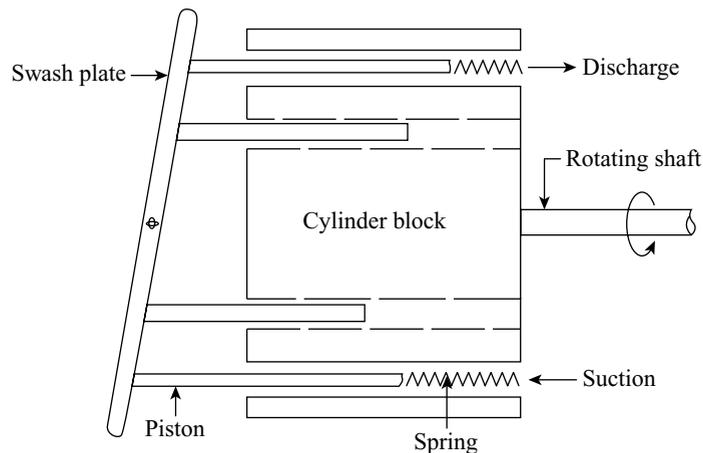
Figure 26.15 Axial piston pump
