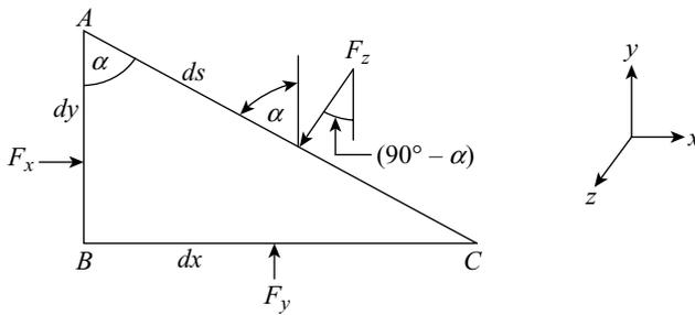
**Figure 2.2** Forces on a static fluid element
