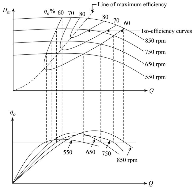
Figure 25.21 Constant efficiency curves
