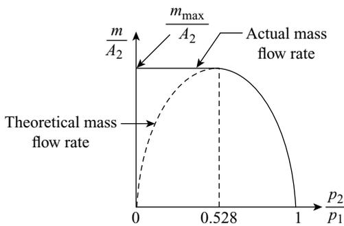
**Figure 17.5** Variation of mass flow rate versus pressure ratio
