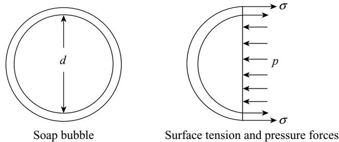
Figure 1.14 Pressure inside the soap bubble
