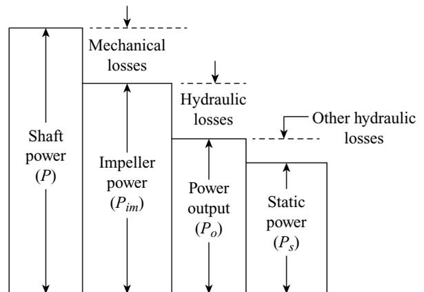
Figure 25.8 Losses in centrifugal pumps
