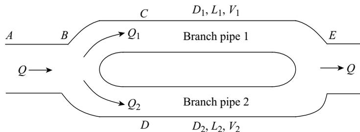
**Figure 14.14** Pipes in parallel
