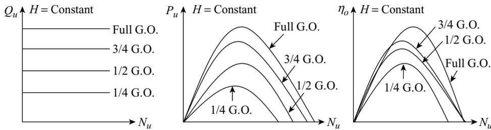
Figure 24.1 Main characteristic curves for the Pelton turbine
