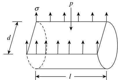
Figure 1.15 Pressure inside a liquid jet
