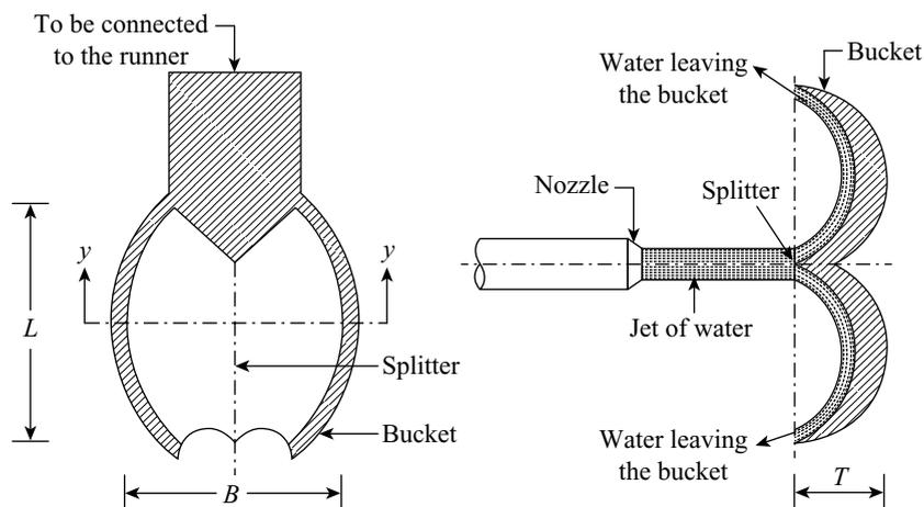
**Figure 21.5** Bucket of Pelton turbine
