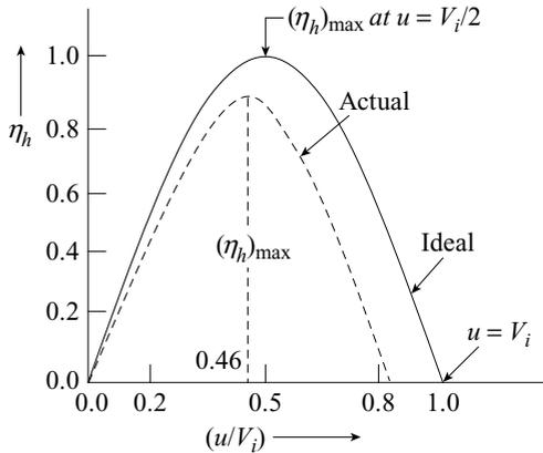
**Figure 21.8** Hydraulic efficiency versus speed ratio
