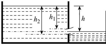
**Figure 10.8** Partially submerged orifice
