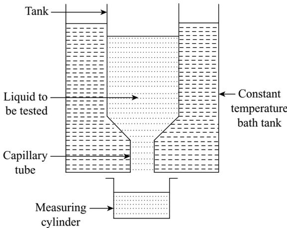
Figure 12.22 Saybolt viscometer
