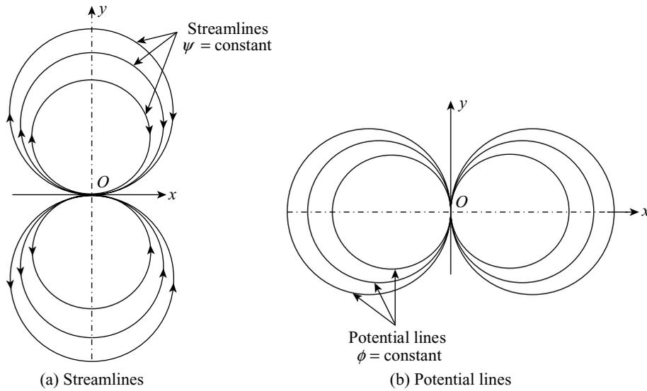
**Figure 9.18** Streamlines and potential lines for a doublet
