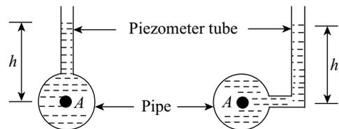
Figure 2.6 Piezometers
