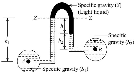
Figure 2.25 Inverted U-tube differential manometer
