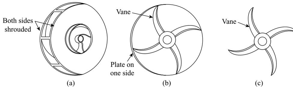
**Figure 25.4** *Types of Impeller*
