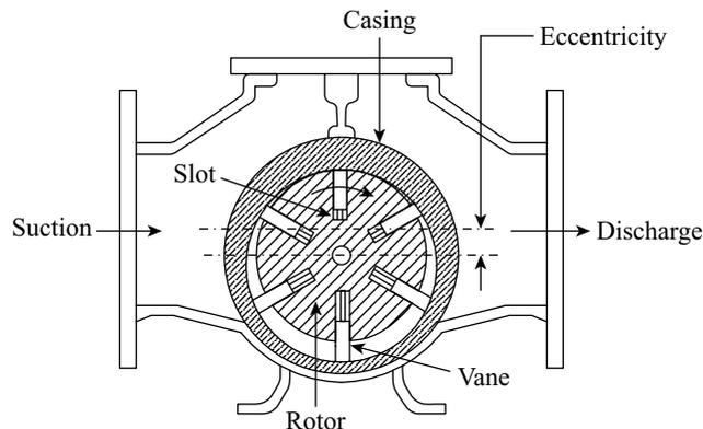
Figure 26.13 Vane pump
