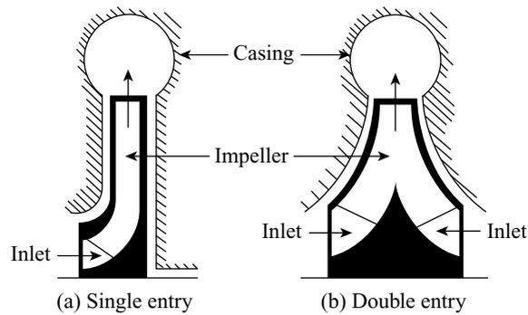
**Figure 25.2** *Single and double suction pumps*
