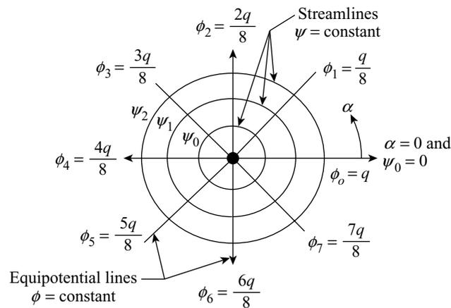
**Figure 9.8** Streamlines and equipotential lines for a free vortex flow
