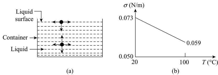
**Figure 1.12** (a) Surface tension (b) Surface tension of water versus temperature
