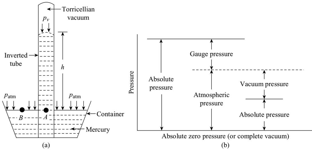
**Figure 2.5** (a) A barometer (b) The scale of pressure
