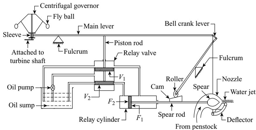
Figure 21.6 Governing mechanism of Pelton turbine
