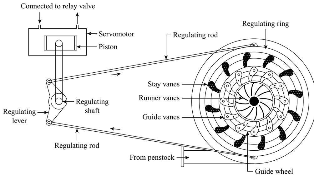
**Figure 22.6** Governing mechanism of Francis turbine
