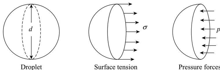
**Figure 1.13** Pressure inside the liquid droplet
