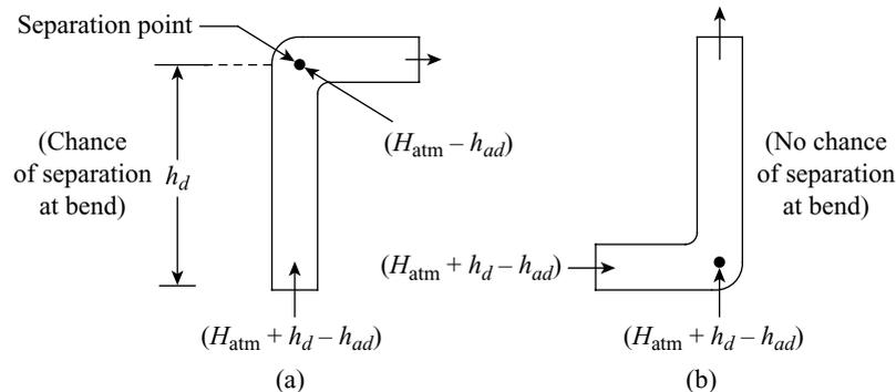
**Figure 26.7** Arrangements of delivery pipes
