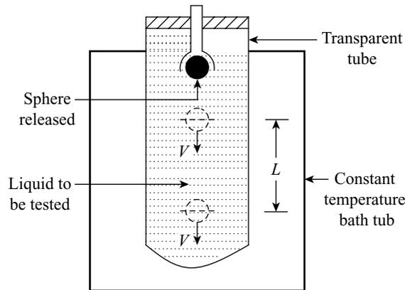
**Figure 12.21** Falling sphere viscometer
