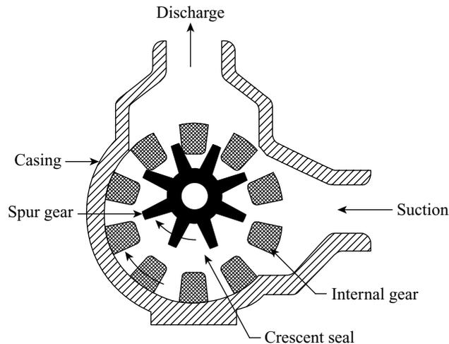
Figure 26.16 Internal gear pump
