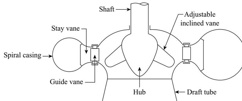
**Figure 23.9** Deriaz (or diagonal) turbine
