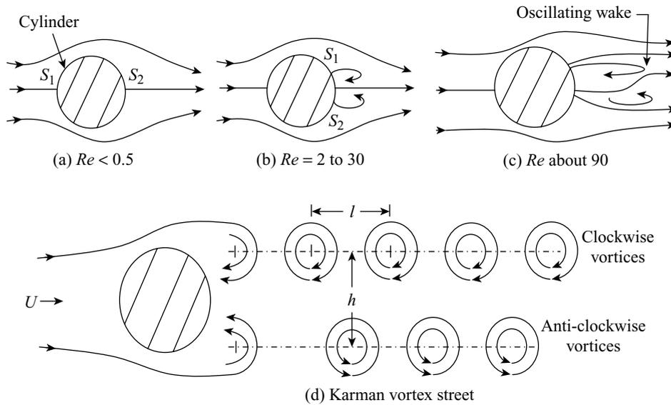
**Figure 16.5** Flow past an infinitely long circular cylinder
