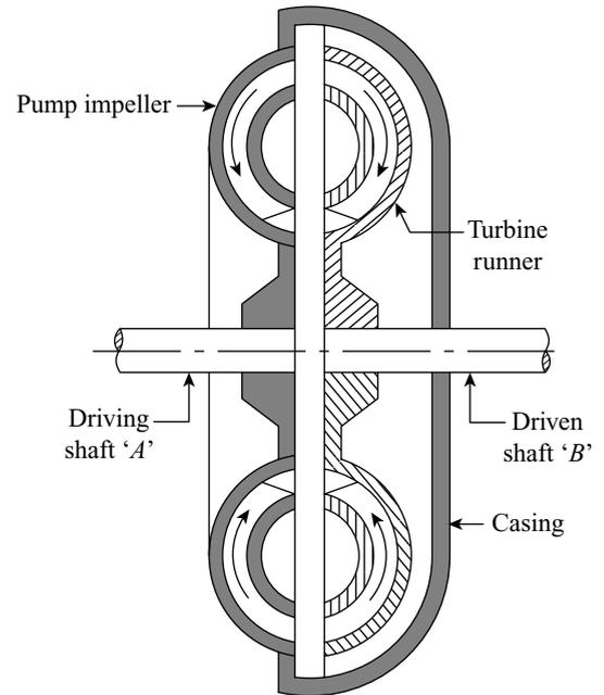
Figure 27.10 Hydraulic coupling
