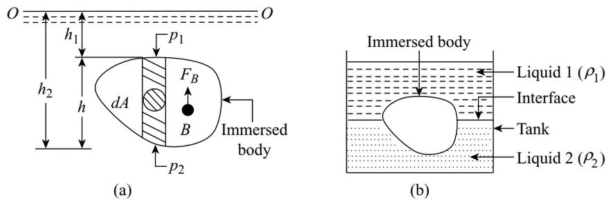
**Figure 5.1** Archimedes' principle
