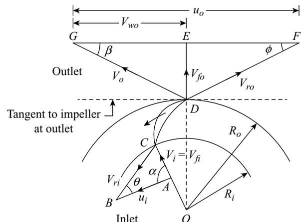
**Figure 25.6** Velocity triangles at inlet and outlet of a centrifugal pump
