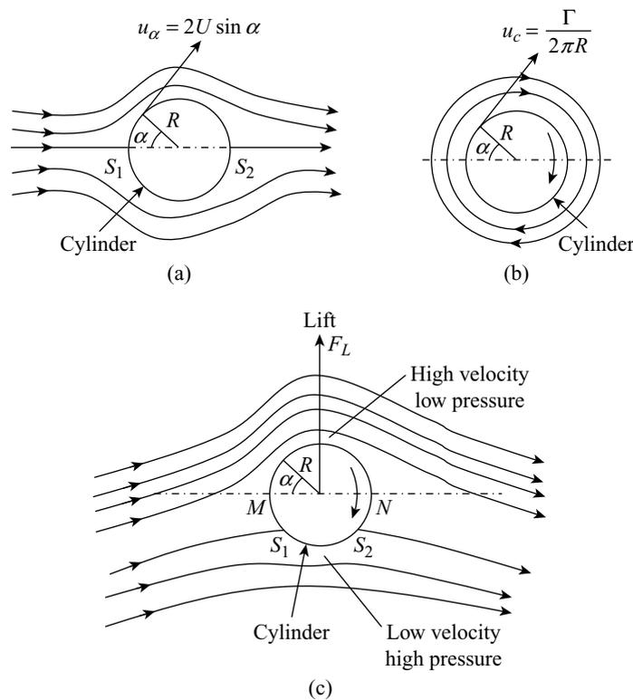
**Figure 16.6** Flow pattern over a stationary and rotating cylinder
