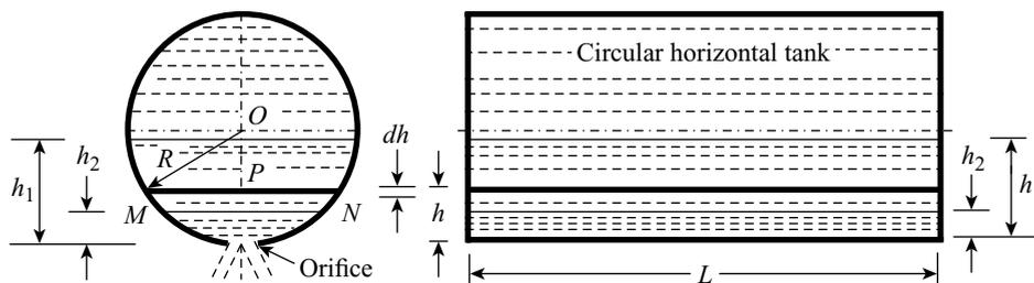
**Figure 10.13** Circular horizontal tank with an orifice at its bottom
