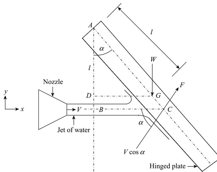
Figure 20.19 Force on a hinged plate
