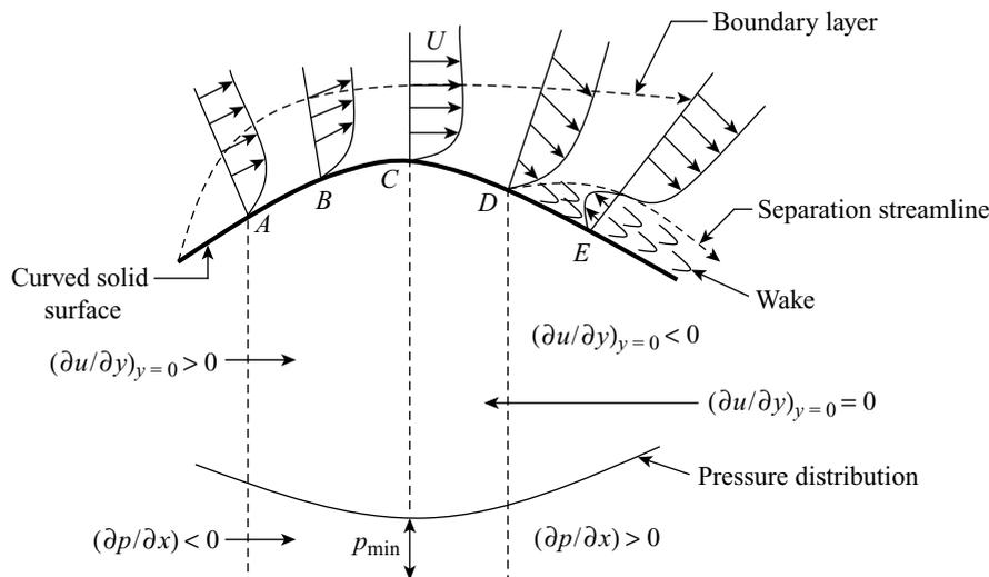
Figure 15.4 Separation of boundary layer
