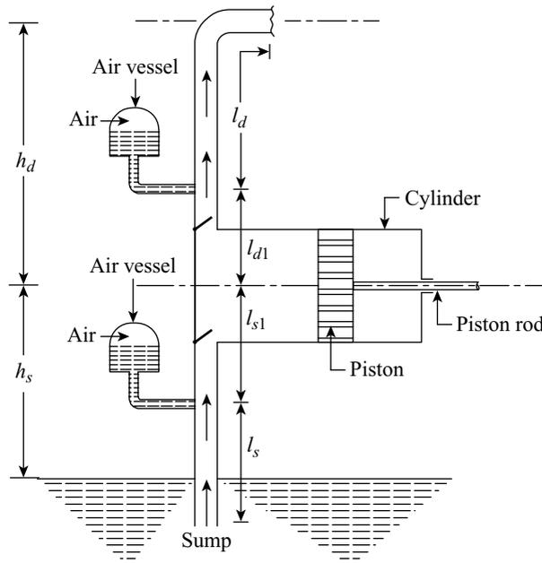
**Figure 26.10** A reciprocating pump with air vessels
