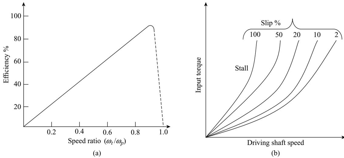
Figure 27.11 Performance characteristics of a hydraulic coupling
