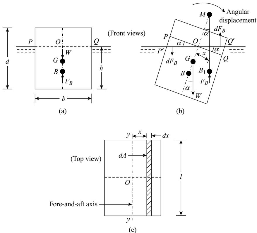
**Figure 5.10** Metacentric height of a floating body
