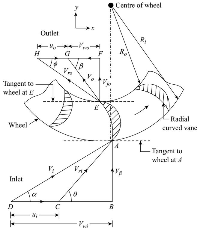
Figure 20.17 Series of curved vanes mounted radially on a wheel
