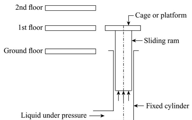
**Figure 27.7** Direct acting hydraulic lift
