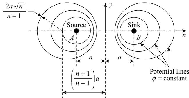
Figure 9.15 Equipotential lines pattern for source-sink pair
