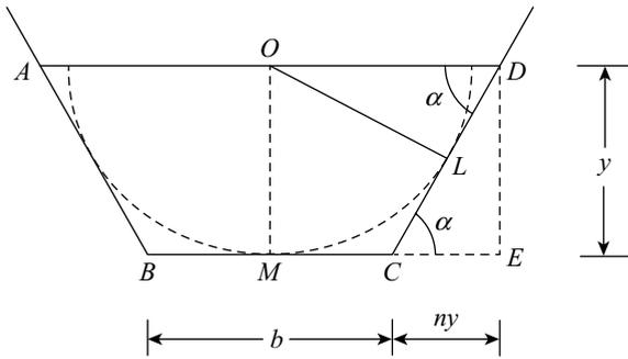
**Figure 18.7** Trapezoidal channel of most economical section
