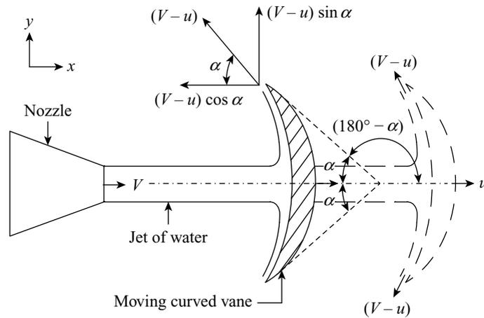
**Figure 20.10** Jet striking a symmetrical curved moving vane at its centre
