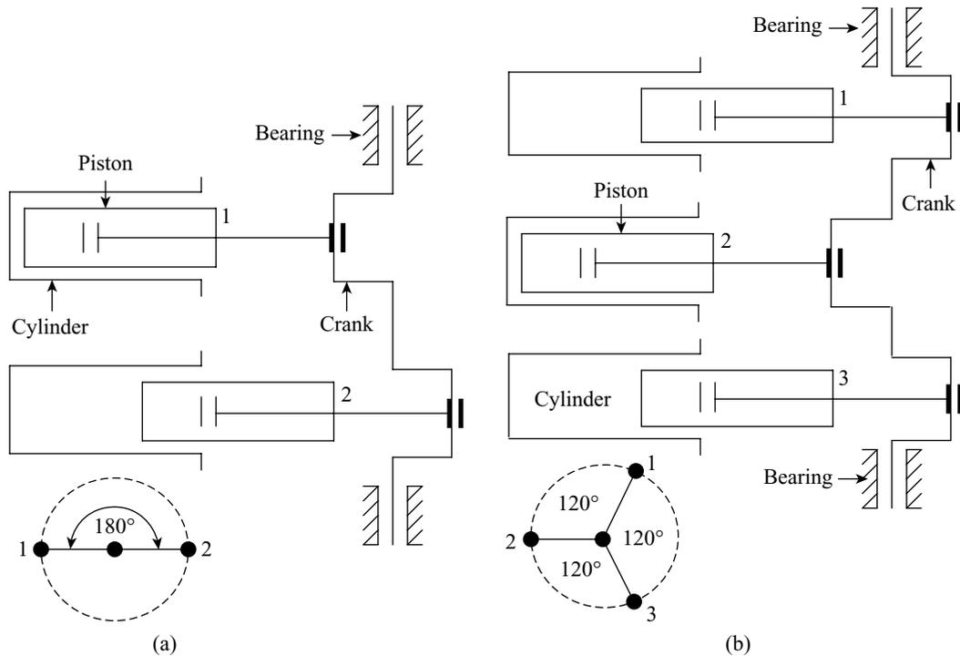
**Figure 26.1** (a) Double cylinder pump (b) Triple cylinder pumps
