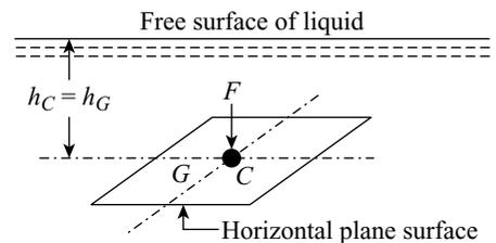
**Figure 3.2** Horizontal submerged plane surface
