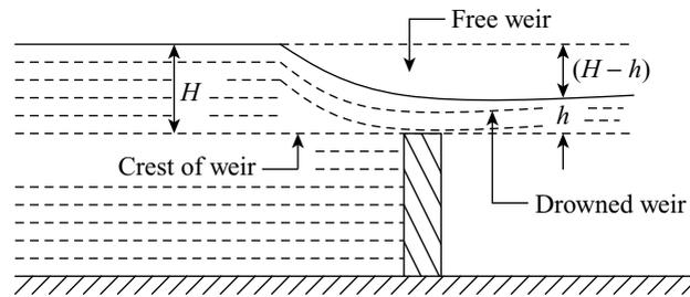
Figure 11.13 Submerged weir
