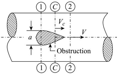
**Figure 14.4** Flow through a pipe having an obstruction
