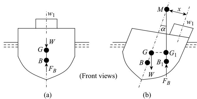
**Figure 5.11** Experimental method for metacentric height of a floating body
