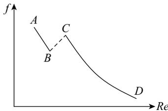
**Figure 13.6** Variation of friction coefficient with Reynolds number
