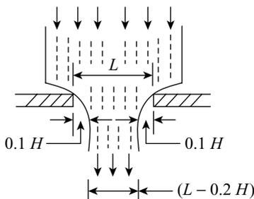
**Figure 11.3** Rectangular weir with end contractions
