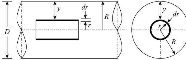
**Figure 13.5** Velocity distribution and forces on control volume in a pipe flow
