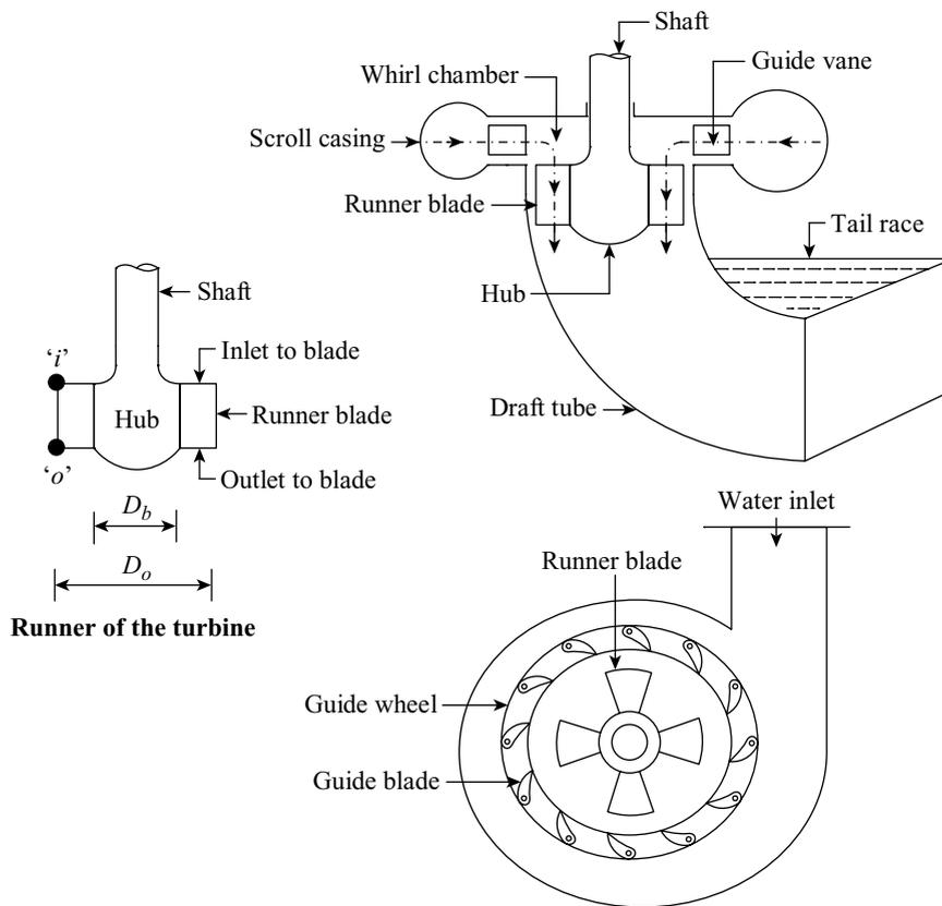
**Figure 23.2** Kaplan turbine and its runner
