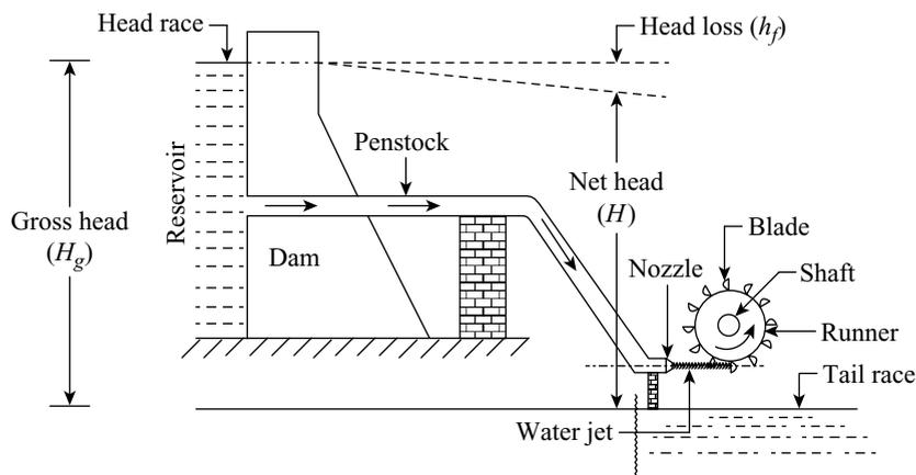
Figure 21.2 General layout of a hydroelectric power plant
