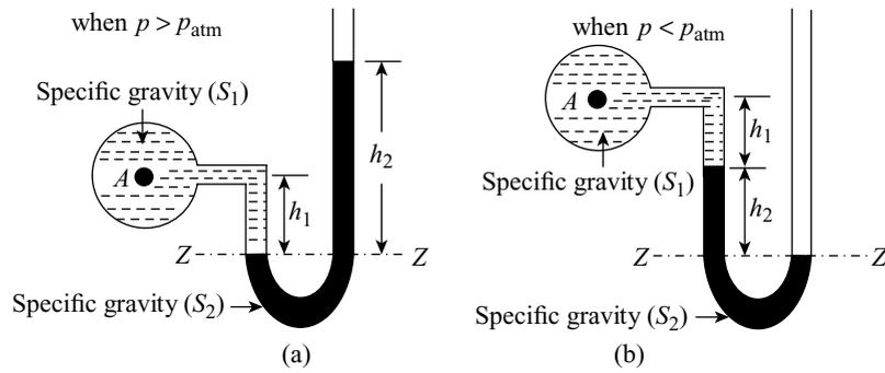
Figure 2.8 U-tube manometers
