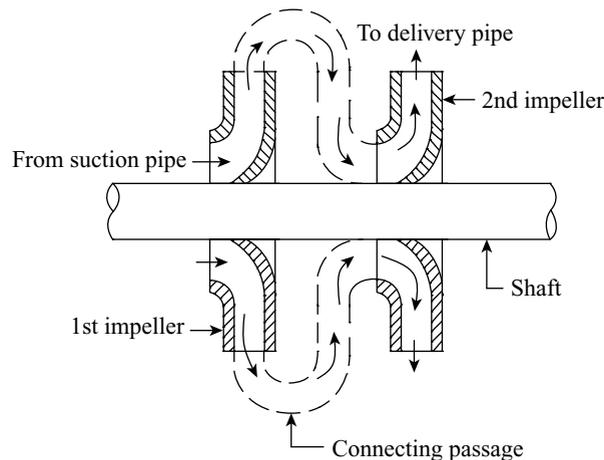
**Figure 25.16** Impellers in series
