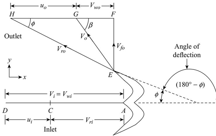
Figure 21.7 Velocity triangles of Pelton turbine
