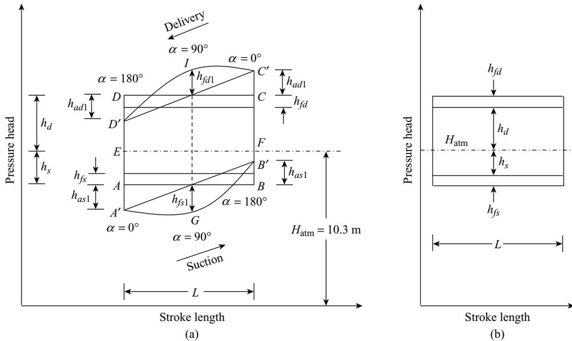
Figure 26.11 Indicator diagram for a reciprocating pump with air vessels
