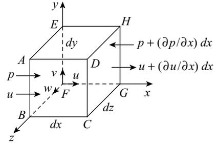
**Figure 12.3** Three-dimensional infinitesimal fluid element
