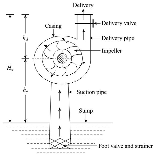
**Figure 25.3** *Main parts of a centrifugal pump*
