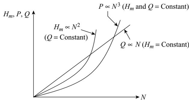
Figure 25.22 Constant head, discharge, and power curves
