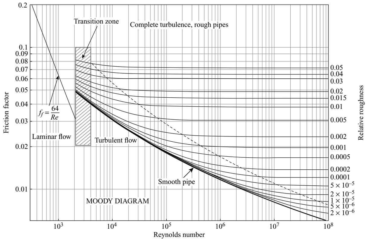
Figure 13.7 Moody diagram for friction factor
