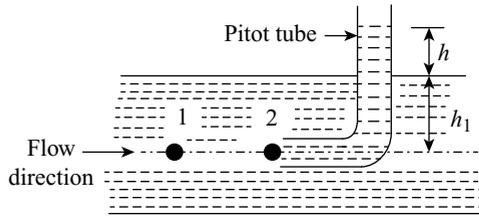
Figure 7.12 Simple pitot tube
