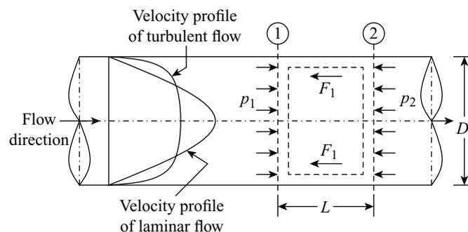
**Figure 13.1** Velocity distribution and forces on control volume in a pipe flow
