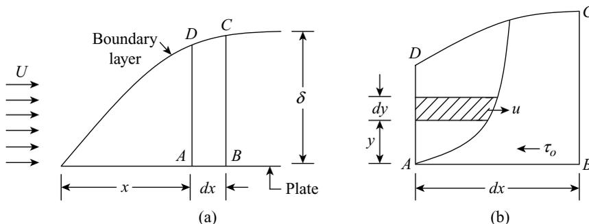
Figure 15.3 Drag force on a flat plate
