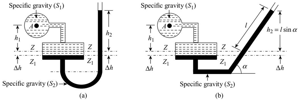
**Figure 2.14** (a) vertical single column manometer (b) inclined single column manometer
