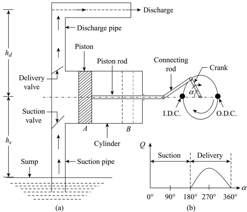
**Figure 26.2** (a) Main parts of a reciprocating pump (b) Variation of discharge
