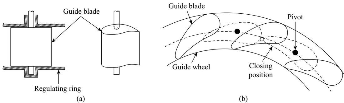
**Figure 22.5** Guide vanes and guide wheel
