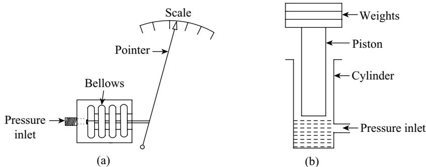
Figure 2.31 (a) Bellows pressure gauge (b) Dead weight pressure gauge
