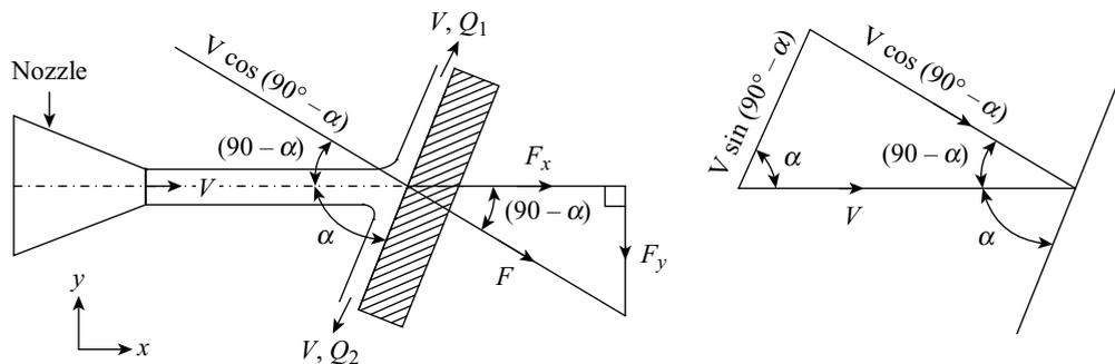
**Figure 20.3** Jet striking an inclined stationary flat plate
