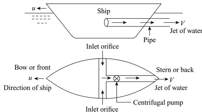
**Figure 20.22** Inlet orifices at right angle to the motion of the ship
