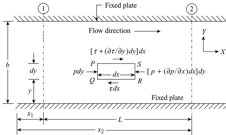
**Figure 12.10** Laminar flow between two parallel fixed plates
