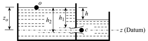
**Figure 10.7** Fully submerged orifice
