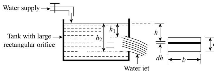
Figure 10.6 Large rectangular orifice
