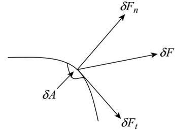
Figure 1.1 Normal and shear forces
