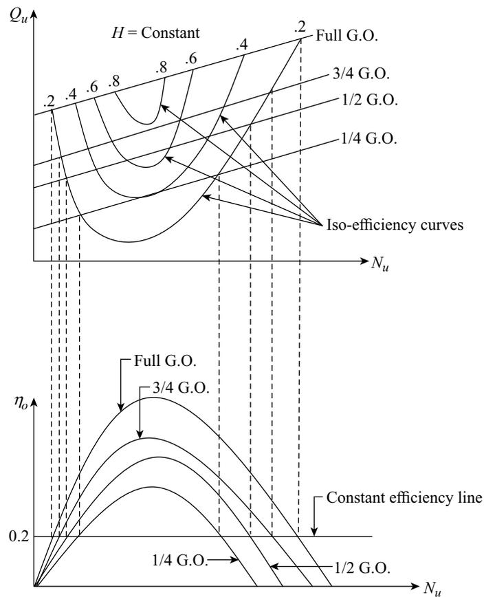
**Figure 24.4** Constant efficiency curves
