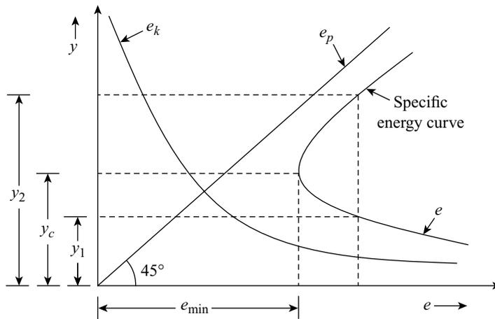
Figure 18.9 Specific energy curve
