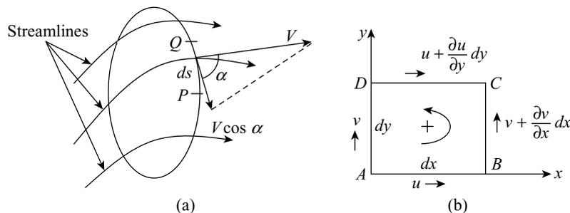
**Figure 6.11** Circulation around (a) closed curve (b) an infinitesimal rectangle
