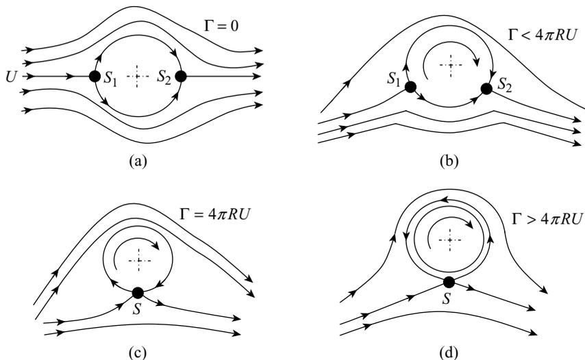
**Figure 9.25** Flow pattern over a rotating circular cylinder
