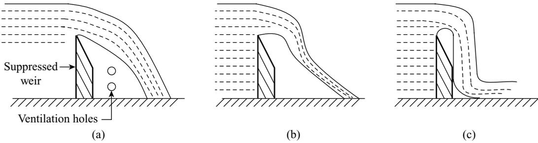
Figure 11.14 Types of nappe over a suppressed weir
