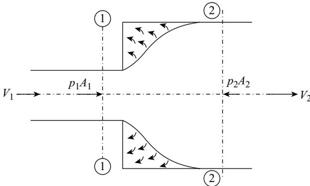
Figure 14.1 Sudden enlargement in a pipe
