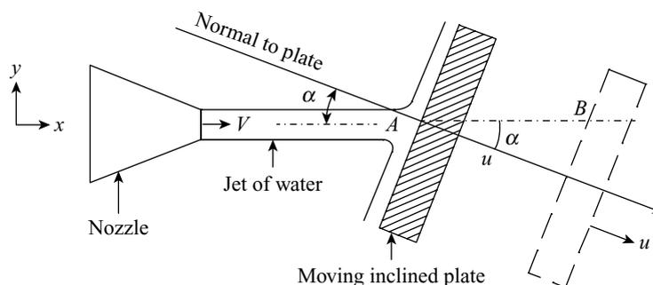
**Figure 20.5** Jet striking to moving inclined flat plate parallel to itself
