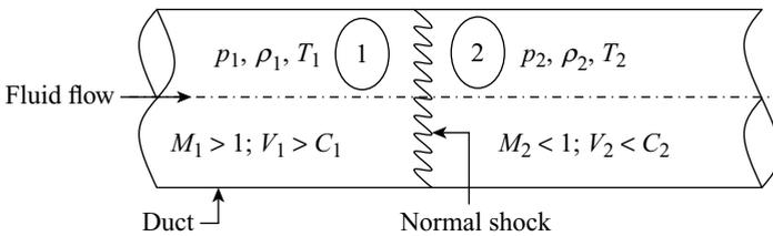
Figure 17.7 Normal shock wave
