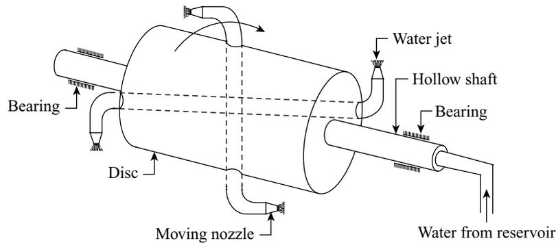
Figure 22.1 Operation principle of reaction turbine
