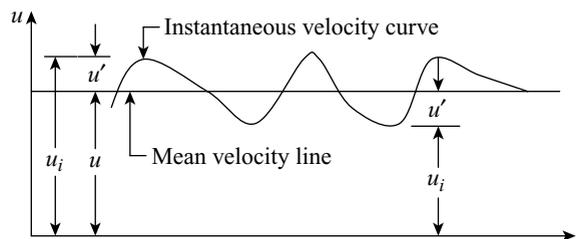
Figure 13.2 Mean and fluctuating velocities
