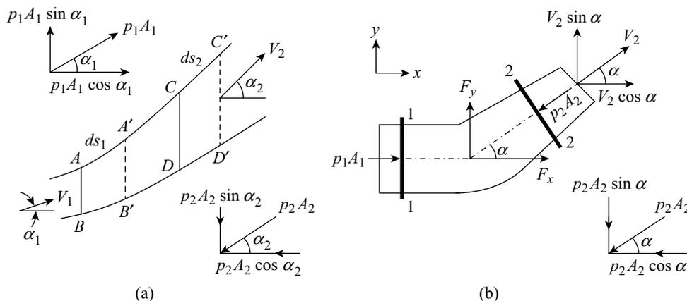
Figure 7.20 Momentum equation for steady flow and force on a pipe bend
