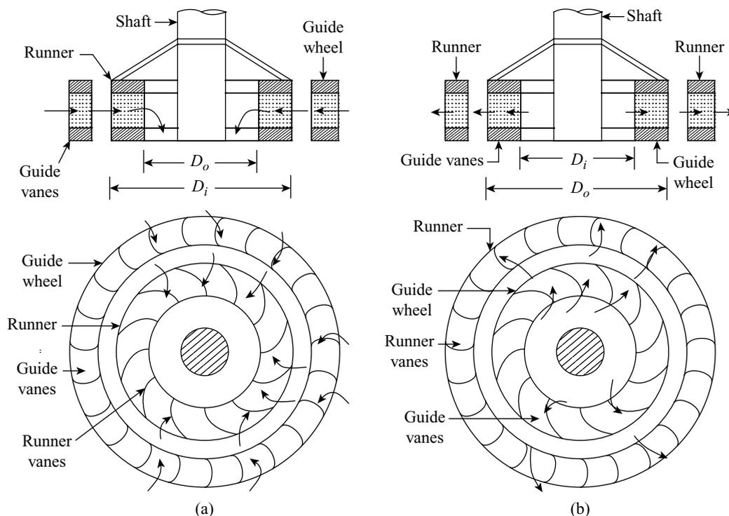
**Figure 22.3** Inward and outward radial flow reaction turbines
