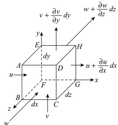
**Figure 6.7** Three-dimensional infinitesimal fluid element
