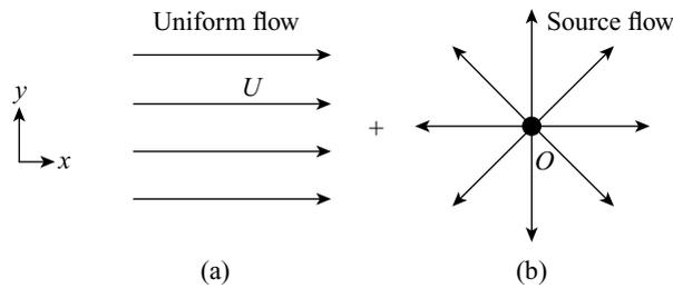
Figure 9.9 (a) Uniform flow (b) Source flow
