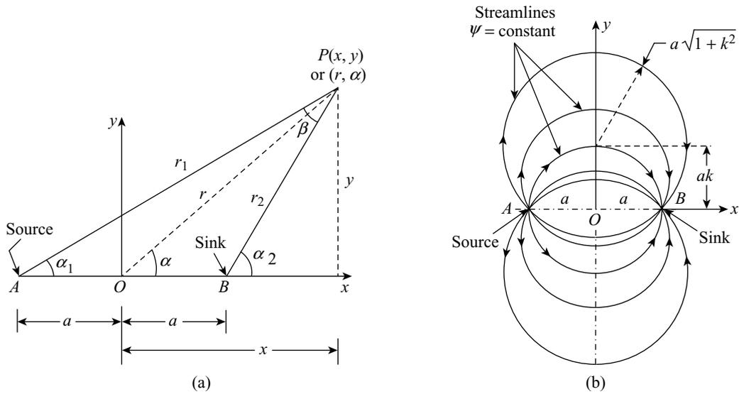
**Figure 9.14** (a) Source-sink pair (b) Streamlines pattern for source-sink pair
