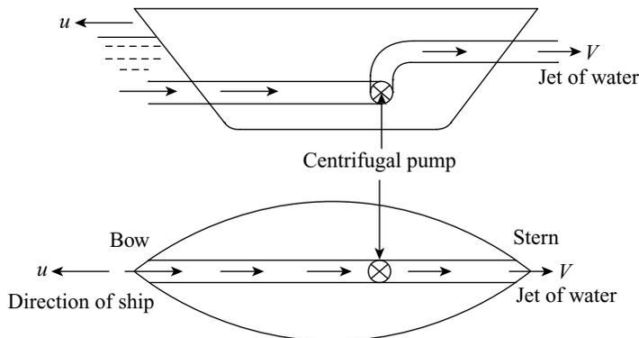
**Figure 20.23** *Inlet orifices face the direction of motion of the ship*
