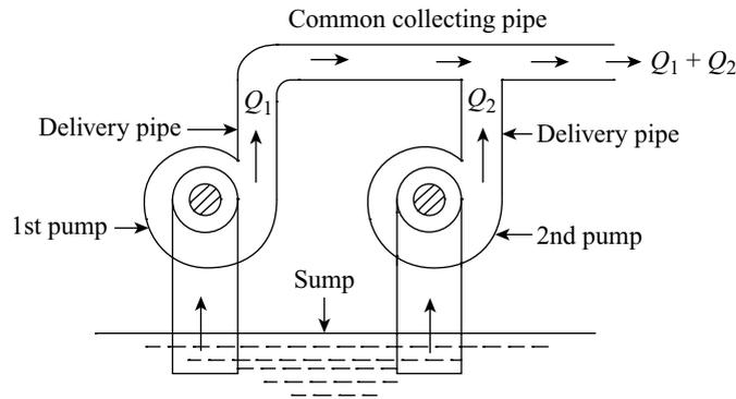
Figure 25.17 Impellers in parallel
