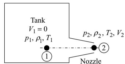
**Figure 17.4** Fluid flow through a convergent nozzle
