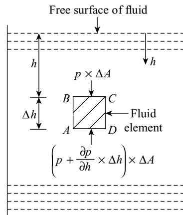
**Figure 2.3** Forces acting on a static fluid element
