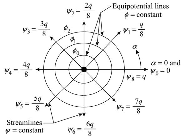
**Figure 9.5** Streamlines and equipotential lines for a source flow
