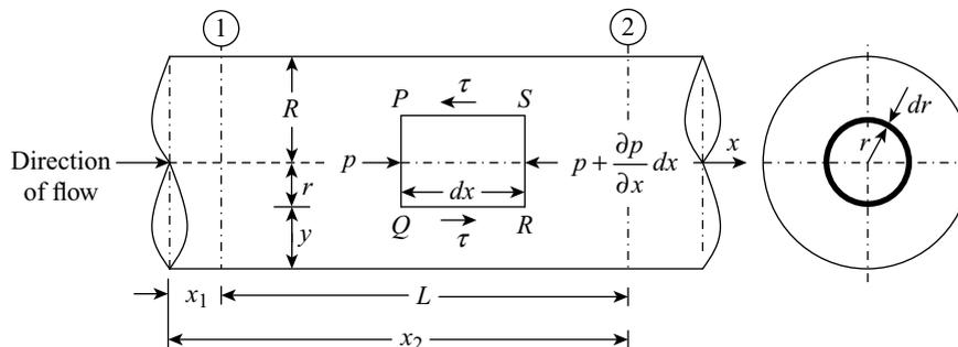
Figure 12.5 Laminar flow through a circular pipe
