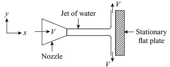
Figure 20.1 Jet striking a stationary vertical flat plate
