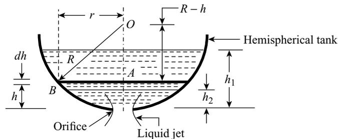
Figure 10.11 Hemispherical tank with an orifice at its bottom
