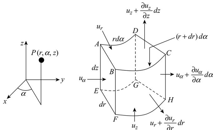
Figure 6.8 Three-dimensional infinitesimal cylindrical fluid element
