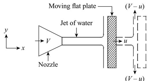
Figure 20.2 Jet striking a vertical flat moving plate
