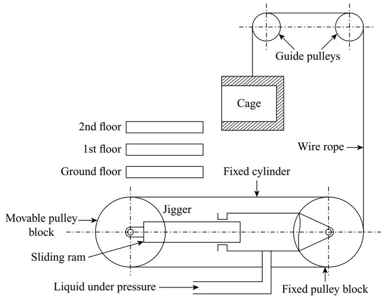
**Figure 27.8** Suspended hydraulic lift
