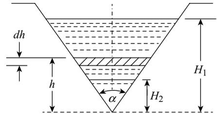
**Figure 11.16** Emptying a reservoir by a triangular weir or notch
