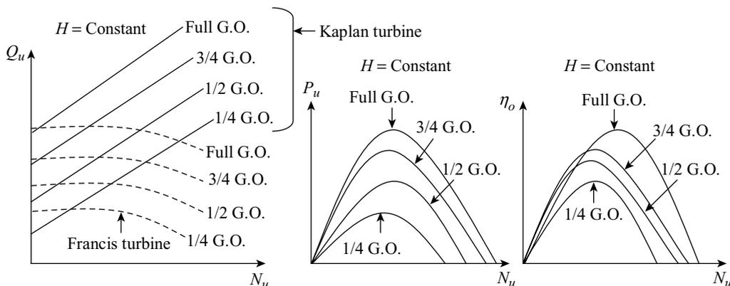
Figure 24.2 Main characteristic curves for reaction turbines
