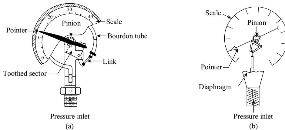
Figure 2.30 (a) Bourdon tube pressure gauge (b) Diaphragm pressure gauge
