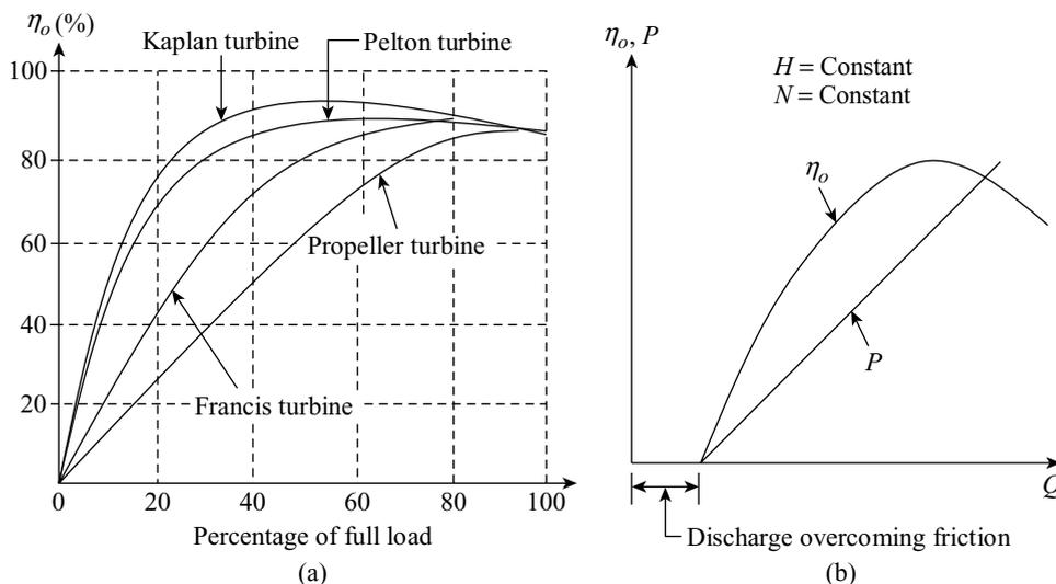
Figure 24.3 Operating characteristic curves
