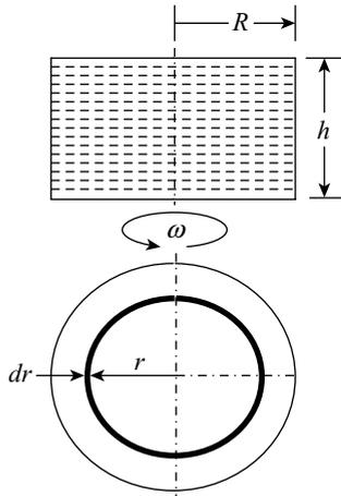
**Figure 8.9** Rotation of a closed cylinder completely filled with a liquid
