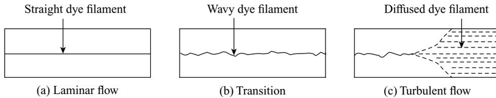
**Figure 12.2** Stages of dye filament
