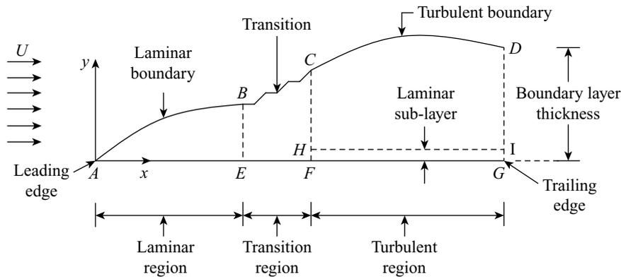
**Figure 15.1** Boundary layer for flow over a flat plate and different flow regime
