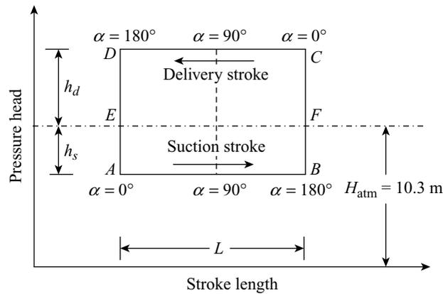
**Figure 26.5** Theoretical (or ideal) indicator diagram
