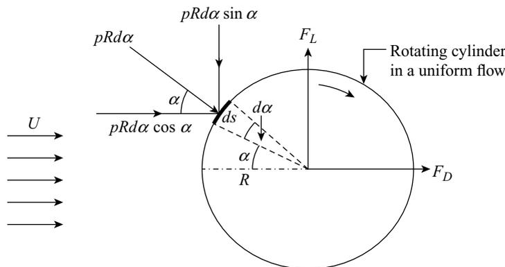
**Figure 16.8** Lift on a rotating cylinder
