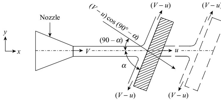
**Figure 20.4** Jet striking to an inclined moving flat plate
