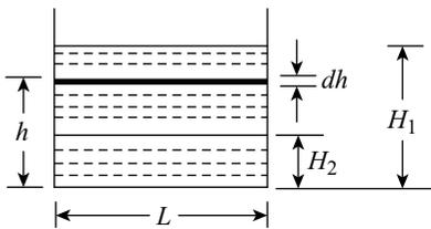
Figure 11.15 Emptying a reservoir by a rectangular weir or notch
