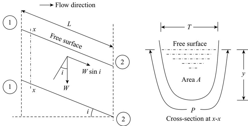
**Figure 18.1** Uniform flow in an open channel
