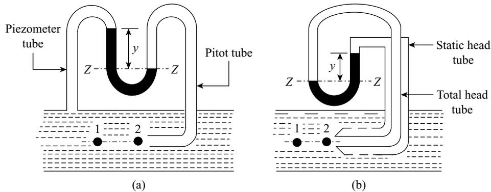
Figure 7.13 (a) Pitot tube (b) Pitot-static tube
