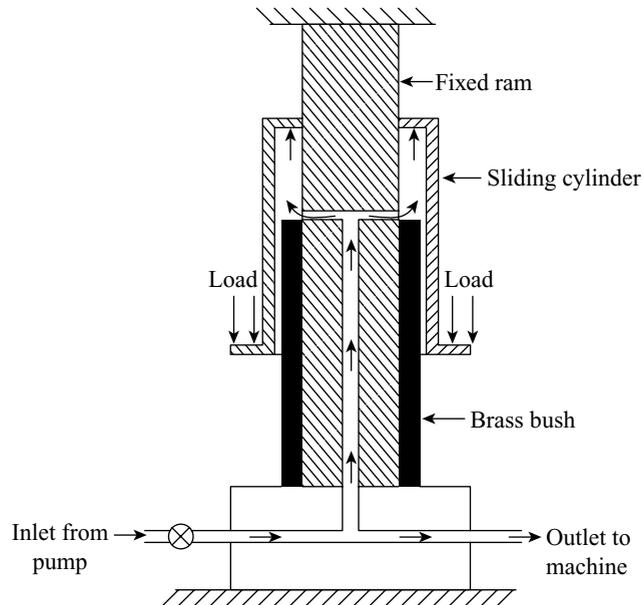
**Figure 27.4** Differential hydraulic accumulator
