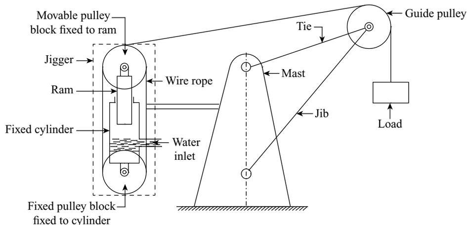
**Figure 27.9** Hydraulic crane
