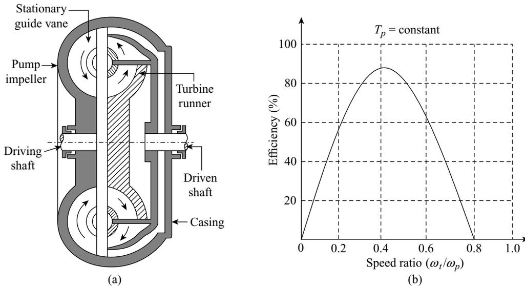
Figure 27.12 Hydraulic torque converter and its characteristics
