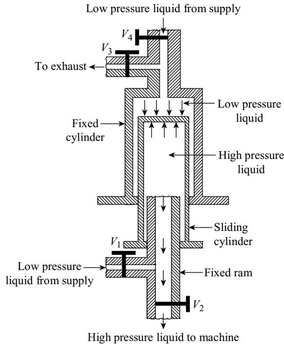
**Figure 27.5** Hydraulic intensifier
