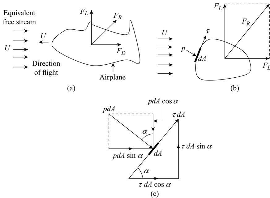
Figure 16.1 Drag and lift forces
