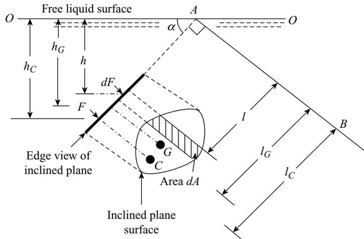
Figure 3.19 Inclined submerged plane surface
