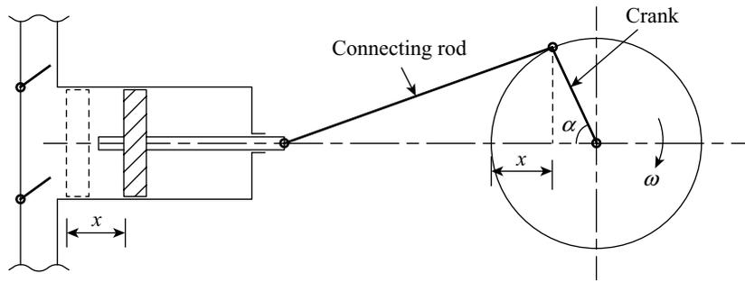
**Figure 26.4** Schematics of single cylinder single acting reciprocating pump
