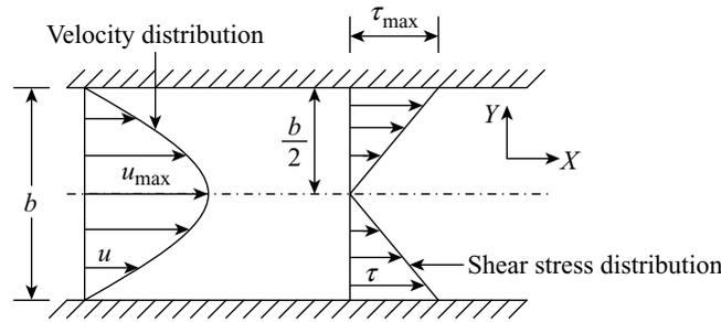
**Figure 12.11** Velocity distribution and shear stress distribution
