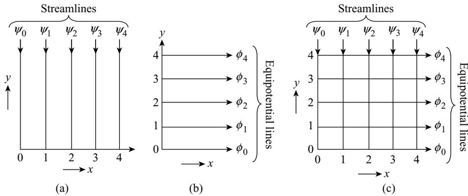
Figure 9.3 Uniform flow parallel to y-axis
