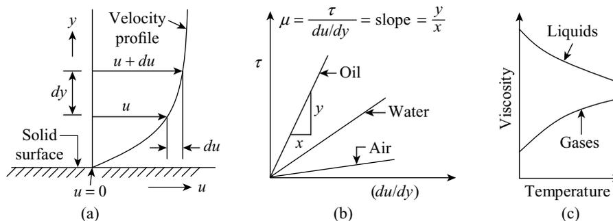
**Figure 1.2** (a) velocity profile (b) shear stress versus velocity gradient (c) viscosity versus temperature
