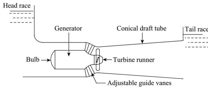
**Figure 23.11** Bulb turbine
