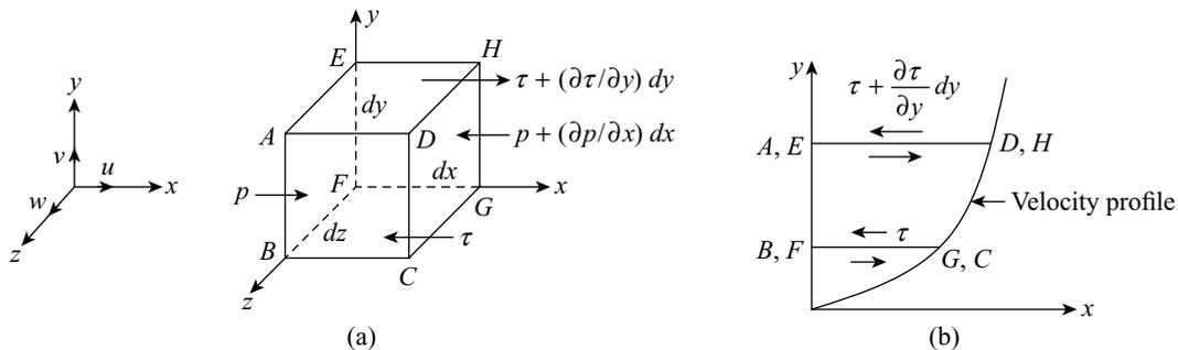
**Figure 12.4** Forces on a fluid element in laminar flow
