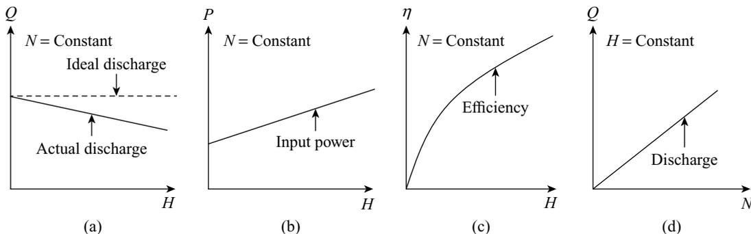
Figure 26.12 Operating characteristic curves of a reciprocating pump
