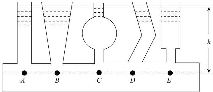
**Figure 2.4** Fluid pressure is same at all points on a horizontal plane
