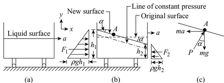
Figure 4.1 Liquid under constant horizontal acceleration
