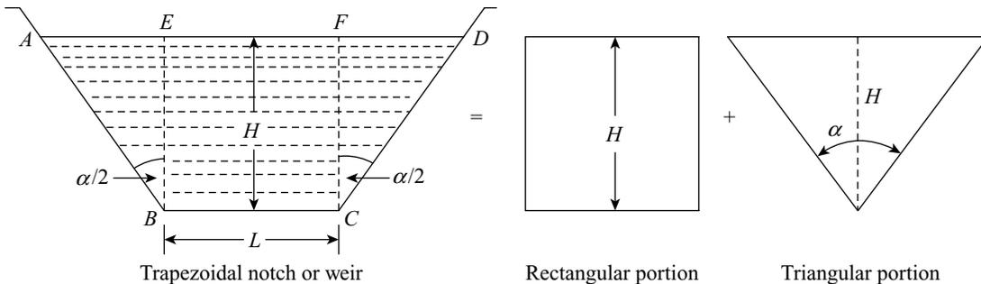
Figure 11.7 Discharge from a trapezoidal notch or weir
