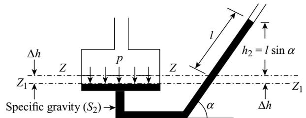
**Figure 2.16****2.7.4 Double U-tube Manometer (Compound Manometer)**
