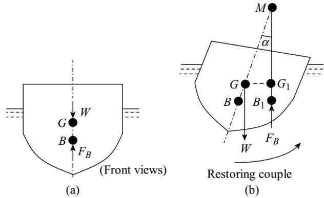
Figure 5.29 Oscillation of a floating body
