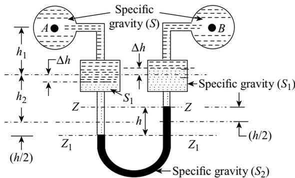
Figure 2.29 Micromanometer
