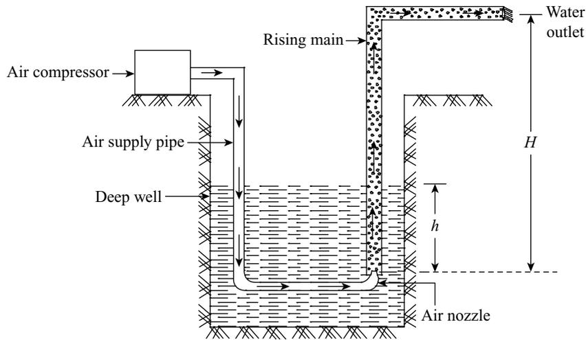
**Figure 27.13** Air lift pump
