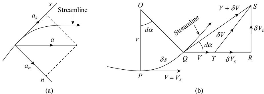
**Figure 6.4** Tangential and normal accelerations
