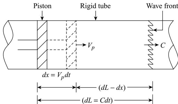
Figure 17.1 Pressure wave propagation
