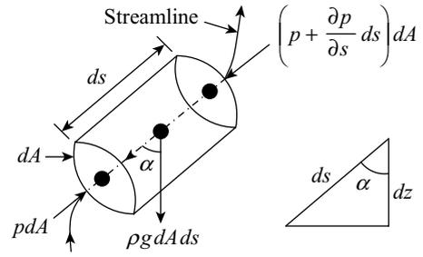
**Figure 7.1** Forces on a fluid element (Euler's equation)
