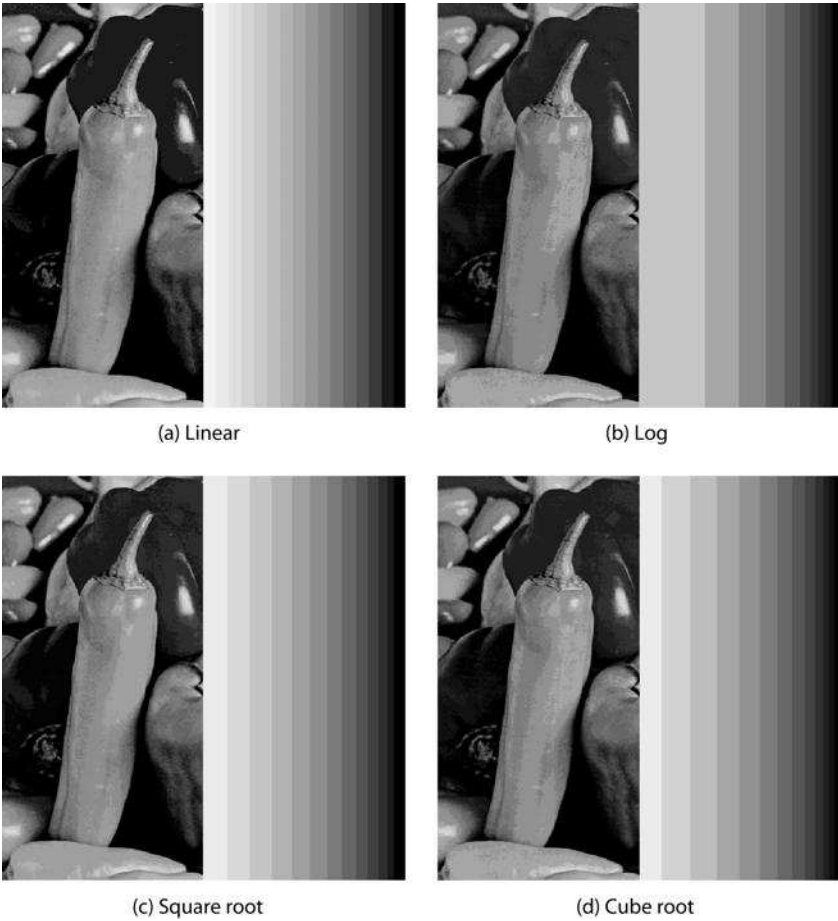
FIGURE 5.3-3. Comparison of lightness scale quantization of the peppers_ramp_luminance image for 4 bit quantization.
