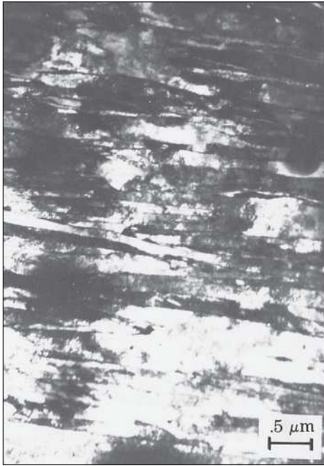
Figure 9.15 Structure of lath martensite in an Fe–0.2% C alloy. (Note the parallel alignment of the laths.) (©ASM International)
