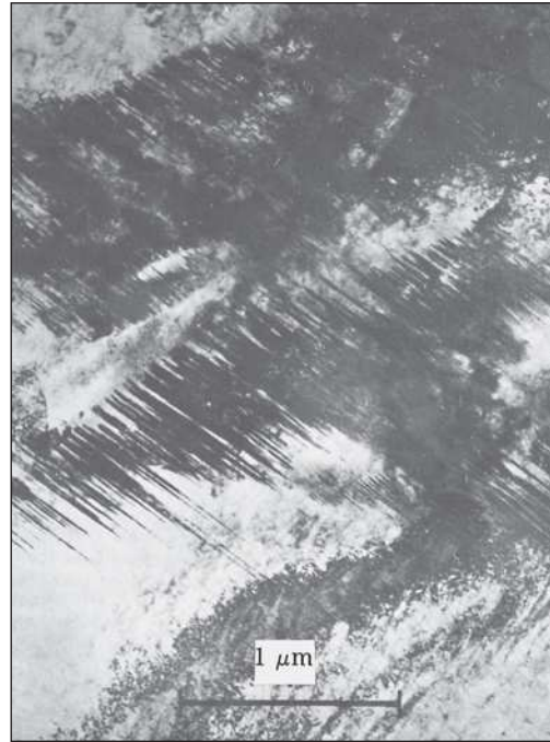
Figure 9.16 Plate martensite showing fine transformation twins. (©ASM International)
