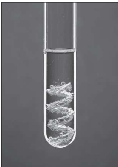
Figure 13.2 Reaction of hydrochloric acid with zinc to produce hydrogen gas. (©GIPhotoStock/Science Source)
