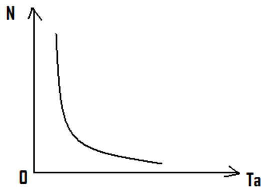
FIG. 7.8 N/T_a Characteristic of a series motor
