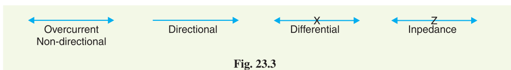
Fig. 23.3 shows the symbols indicating the various types of relays.
