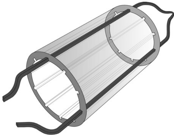
Fig. 5.4 Cylindrical magnetic circuit of a stator containing one turn composed of two conductors laid in the opposite slots
