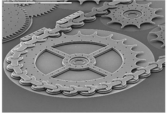
Fig. 13 Detail of Microchain Link and Sprocket: A silicon microchain rather than a silicon microbelt is used in this MEMS because a silicon belt would have spring-like characteristics which would apply too much torque on any sprockets not aligned in the same plane. By contrast, each chain link is capable of \pm 52^\circ rotation with respect to the preceding link. This minimizes stress on the support structure. The longest span unsupported by sprockets or bracing is 500 microns, but a microchain tensioner permits longer spans. This multilevel surface-micromachined device was constructed with Sandia's SUMMIT IV and SUMMIT V technology.
