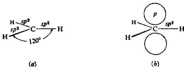
Figure 2.9. Methyl radical. (a) Only \sigma bonds shown. (b) Odd electron in p orbital above and below plane of \sigma bonds.
