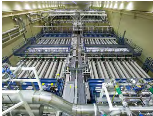
Figure 32.23 National Ignition Facility (CA). This image shows a laser bay where 192 laser beams will focus onto a small D-T target, producing fusion. (credit: Lawrence Livermore National Laboratory, Lawrence Livermore National Security, LLC, and the Department of Energy)
