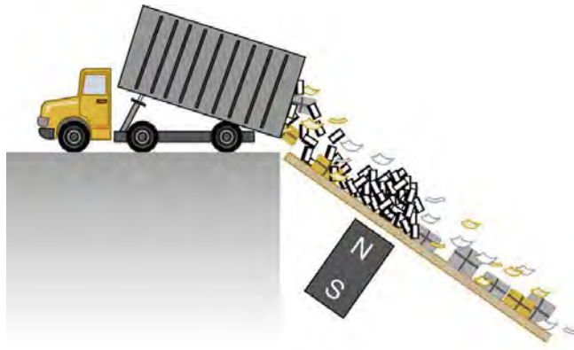
Figure 23.17 Metals can be separated from other trash by magnetic drag. Eddy currents and magnetic drag are created in the metals sent down this ramp by the powerful magnet beneath it. Nonmetals move on.
