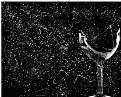
Figure 17.2 This glass has been shattered by a high-intensity sound wave of the same frequency as the resonant frequency of the glass. While the sound is not visible, the effects of the sound prove its existence. (credit: ||read||, Flickr)
