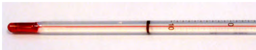
Figure 13.2 In a typical thermometer like this one, the alcohol, with a red dye, expands more rapidly than the glass containing it. When the thermometer's temperature increases, the liquid from the bulb is forced into the narrow tube, producing a large change in the length of the column for a small change in temperature. (credit: Chemical Engineer, Wikimedia Commons)
