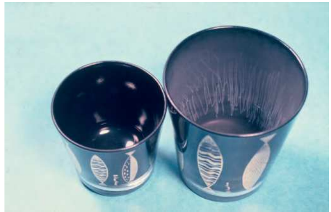
Figure 39-2 Cocktail glasses with the original interior shellac coating (left) removed by dishwasher heat (right), exposing the dull lead-based paint lining (scratches made for sampling analysis).
