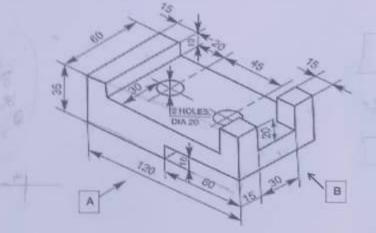
(a) From the given isometric projection shown above, produce a third angle orthographic projection of the component using a scale of 1:2, showing the following details:
