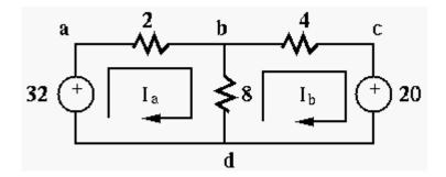
Find currents  $I_1$  from a to b,  $I_2$  from c to b, and  $I_3$  from b to d.
