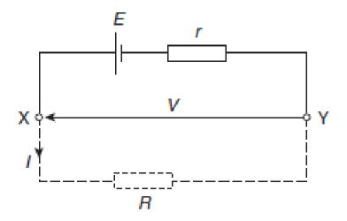
When a load (shown as resistance R) is not connected, no current flows and the terminal p.d., V =E. When R is connected a current I flows which causes a voltage drop in the cell, given by Ir. The p.d. available at the cell terminals is less than the e.m.f. of the cell and is given by V = E - Ir
