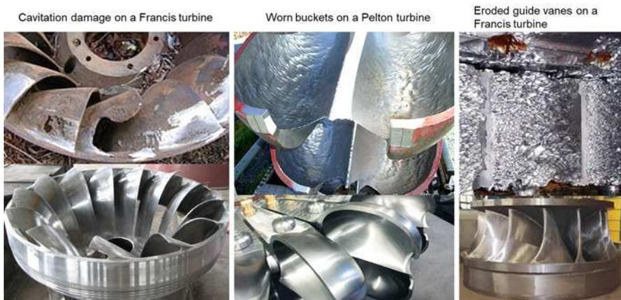
**Fig. 7.4** Typical examples of corrosion and erosion of turbine components (up part is used; bottom part is new-built)
