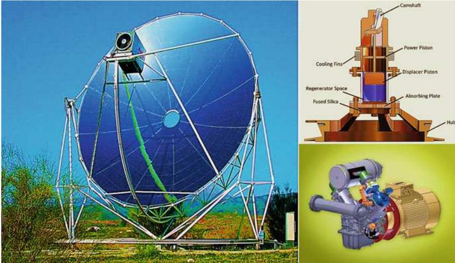
**Fig. 4.8** Solar Stirling engine
