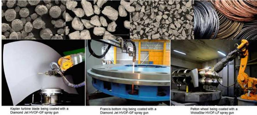
**Fig. 7.5** Examples of coating materials with different morphologies and coating application technologies (Modified from Oerlikon Metco 2014. Courtesy: Oerlikon Metco)
