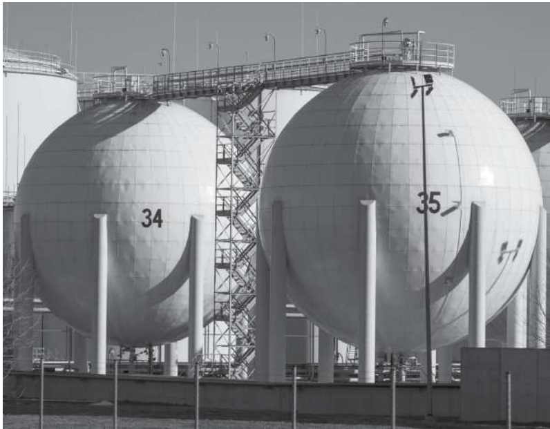
FIGURE 12–2 Examples of pressure vessels. (a) Tanks for propane fuel for home barbecue cooking. (b) Industrial compressor mounted on its integral compressed air storage tank. (c) Large spherical storage tanks for industrial gases.
