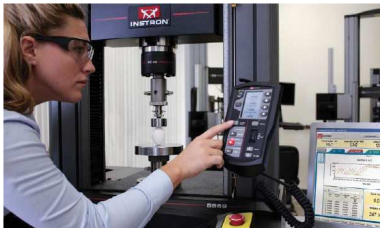
FIGURE 2–1 Understanding the properties of a material is critical to achieving safe and effective designs. Test equipment, such as that shown here, is available to determine the performance of a wide variety of materials with regard to strength and deformation.
