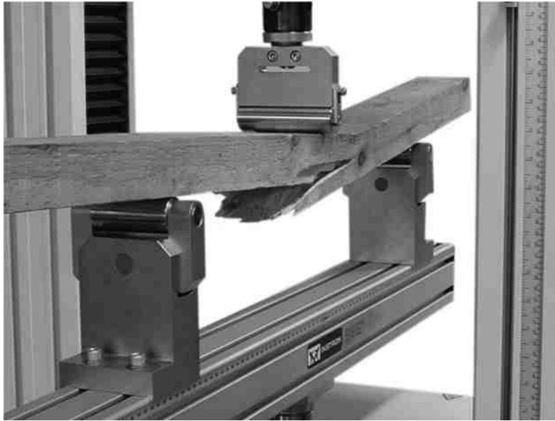
FIGURE 8-1 (See color insert.) Wood beams are particularly susceptible to failure not due to bending stresses as calculated in the last chapter, but instead due to failure in shear. In many applications, designers must take care to analyze shear stress to avoid failures like the one shown in this test fixture.
