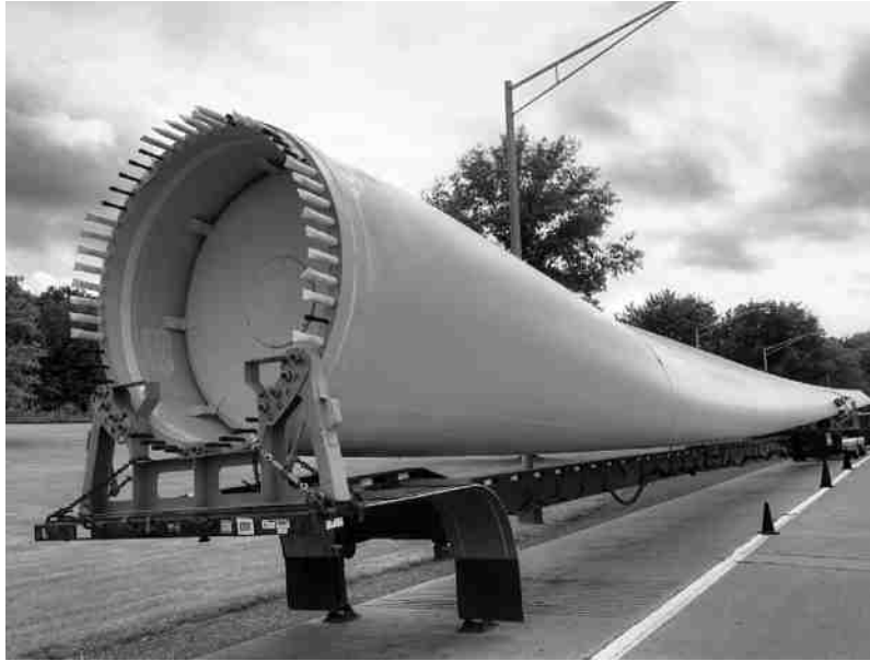
FIGURE 2–22 Large composite wind turbine blade at the installation site.
