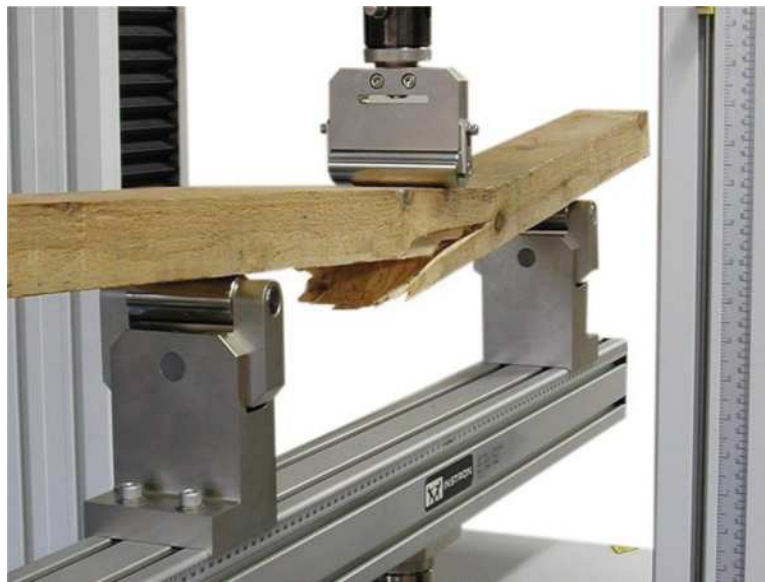
FIGURE 8-1 Wood beams are particularly susceptible to failure not due to bending stresses as calculated in the last chapter, but instead due to failure in shear. In many applications, designers must take care to analyze shear stress to avoid failures like the one shown in this test fixture.
