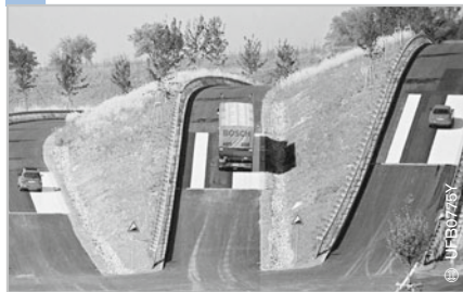
11 Steep uphill drive in the Bosch proving grounds in Boxberg for testing the driving stability systems of passenger cars and commercial vehicles
