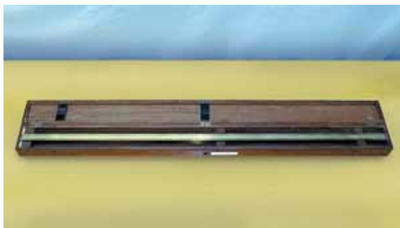
A bar of platinum - iridium metre kept at a temperature of 0° C.
