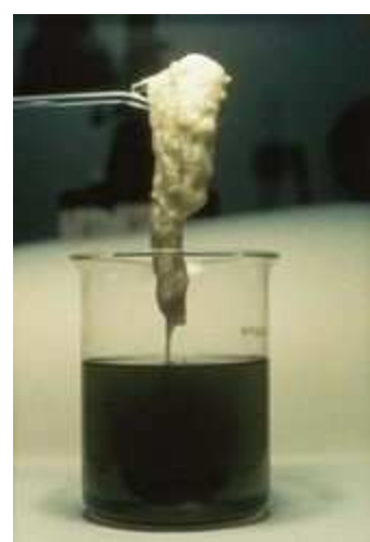
Fig. 28.3 Alcohol extraction of alginate from mucoid Ps. aeruginosa .
