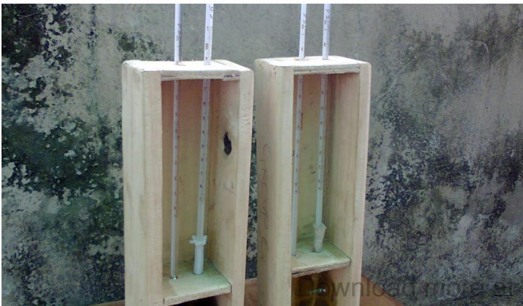
**Figure . Locally constructed Hygrometer**
