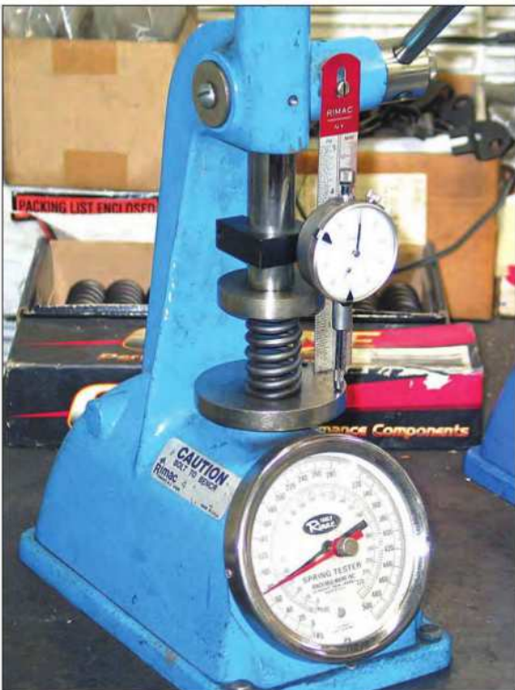
Each valvespring must be checked on a spring tester. The spring is compressed to its specified installed height while recording spring pressure.
