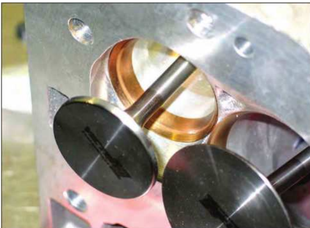
Valve seats for today's aluminum performance heads are, depending on the application, made of ductile iron, silica-bronze, beryllium-copper, powdered metal, or tungsten-carbide. These are silica-bronze seats installed in a Trick Flow cylinder head. Seat material must be compatible with the type of valve material being used.
