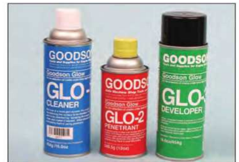
The three-chemical process involves a cleaner/solvent that prepares the surface, a penetrant that seeps into any cracks, and a developer that allows the black light to highlight any cracks.
