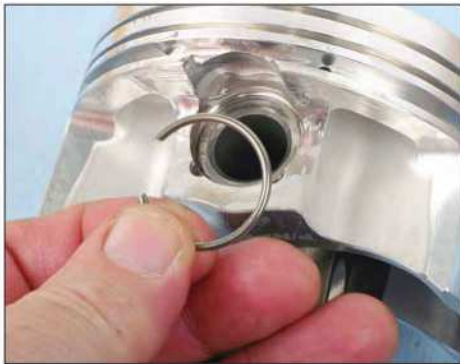
Wire locks are spring steel clips. Insert one end and use your finger or a small drift to walk the clip into its groove.
