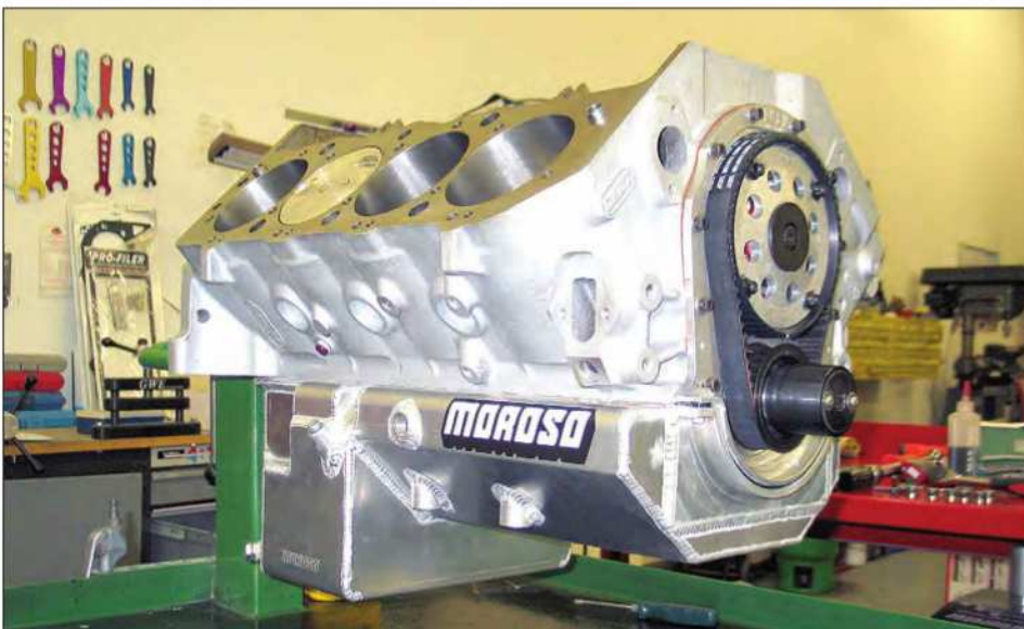
High-performance engines often benefit from a large-capacity custom oil pan. This oversize pan is installed on a Dart Big-M block fitted with a 4.750-inch stroker crank.
