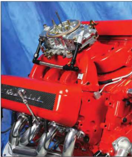
Using the Edelbrock dual-plane intake and a 650-cfm Holley (and a mild-cam change), we simply overbored this 5.3-liter LS iron-block to 327 ci and hit 450 hp. The manifold provided snappy throttle response and favored bottom-end and mid-range power.
