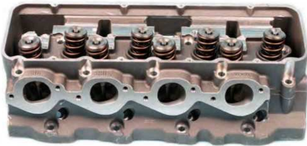
Symmetrical exhaust ports (big-block Chevy pattern on a Dart Big Chief II head).
