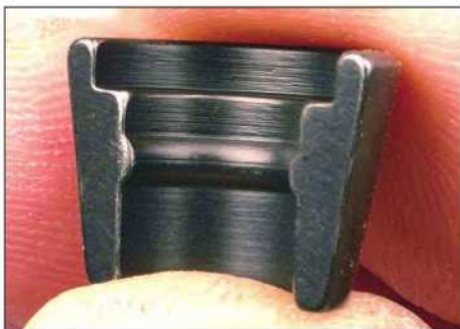
This is a bead-lock valve lock. Remember, this style is only to be used with a bead-lock valve.
