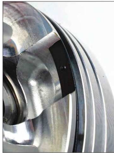
This underside view shows the oil ring support rail properly positioned, with the male dimple centered in the opening above the wrist pin bore. The dimple prevents the support rail from rotating too far (this prevents the support rail gap/ends from moving to an area with no support).
