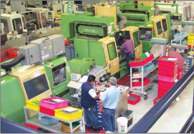
Manufacturers commonly utilize CNC machining for speed of product output and precision results. This shot shows a few of the production CNC machining centers in JE Pistons' facility.
