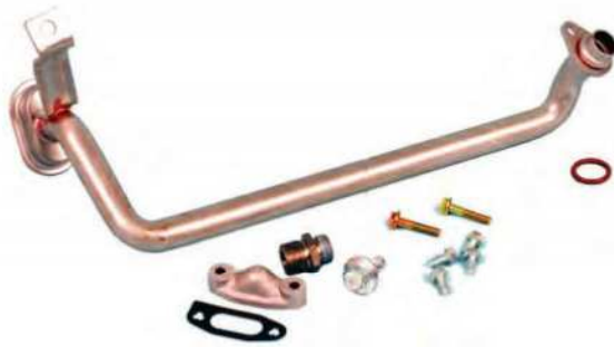
A crank-driven oil pump likely has a lone pickup tube that is necessitated by the location of a rear-pan sump. This type of pump has a pickup tube that bolts to the pump and is sealed with an O-ring, so no interference fitting or welding is needed.
