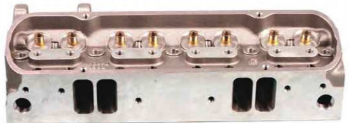
Small-block Ford intake ports. Matching ports to gaskets and heads is critical because of the close proximity of the pairs of ports.
