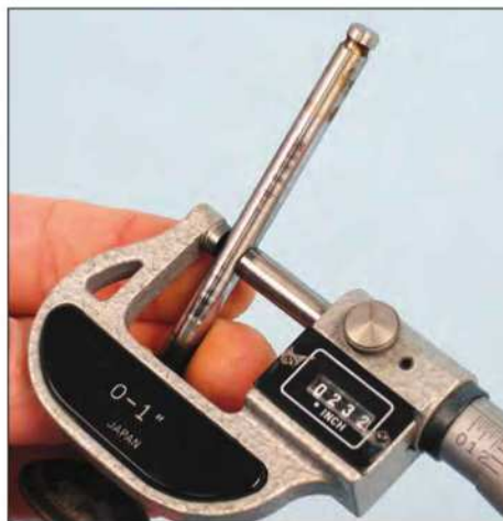
Use a micrometer (not a caliper) to measure valvestem diameter. Take three measurements. Here a stem is measured at its center length area.
