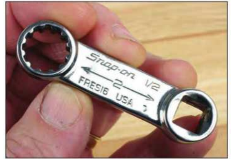
Wrench extensions are readily available from quality tool sources. Just remember to adjust the torque wrench accordingly to compensate for the added leverage.
