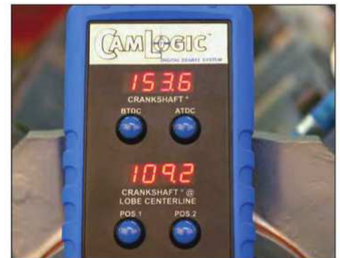
The digital display unit constantly monitors crank angle (top display) and camshaft lobe position (lower display). Using this system is surprisingly simple and quicker than using a degree wheel.
