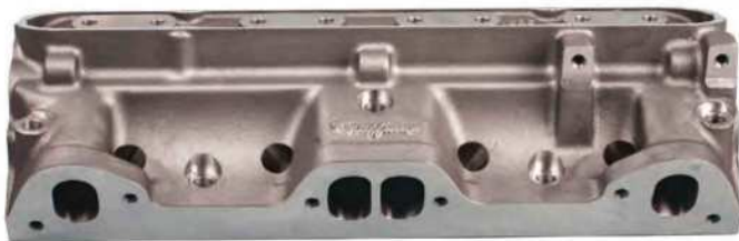
Asymmetrical exhaust ports on a big-block Pontiac head (oval ports at ends and D-ports at center).
