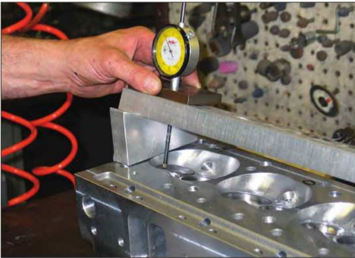
Once initial cuts have been made, valves are installed to check for valve depth. The goal is to establish equal depth of all valves.
