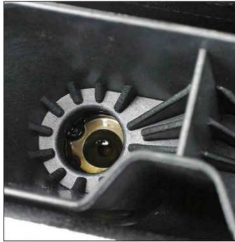
Note the series of small tapered walls in the top of the lifter bucket; they are designed to help drain oil to the lifters. However, this OEM design still tends to hold too much oil and drains slowly. A simple mod involves drilling a couple of 5/16-inch holes around the base of the cavity for faster oil drain.
