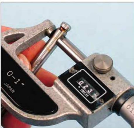
Measure stem diameter just below the lock area.
