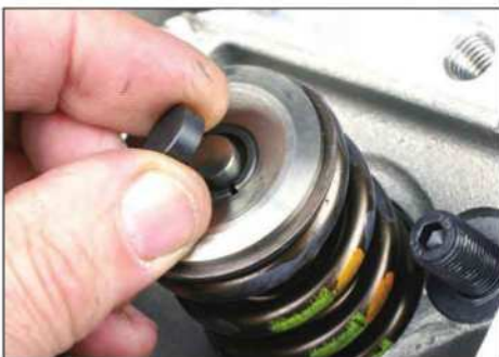
Hardened steel lash caps are designed to protect the relatively soft tip of a titanium valve although titanium valves are now available with built-in hard tips. Lash caps are also useful in fine-tuning rocker arm geometry and valve lash range and are available in various thicknesses. The lash cap should fit snugly onto the valve tip.
