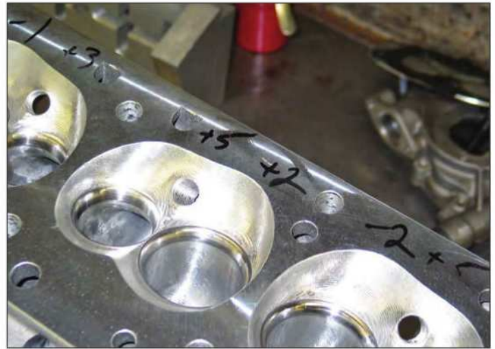
After measuring (and recording) each valve's depth location, finish cuts are made to equalize all valve depths.
