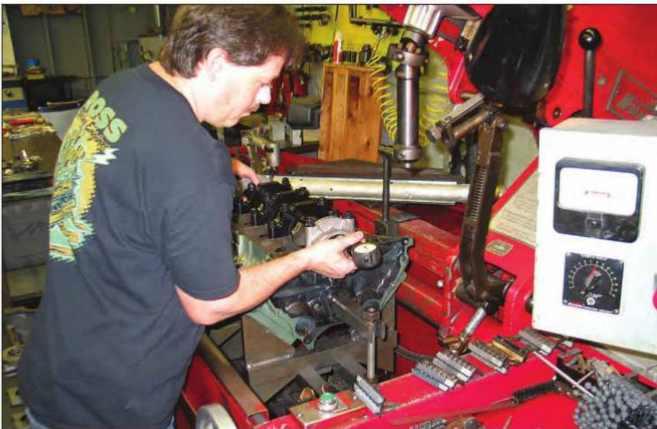
The main bearing journals and caps are honed. After a few passes, the main bore diameters are regularly checked with a precision dial bore gauge.
