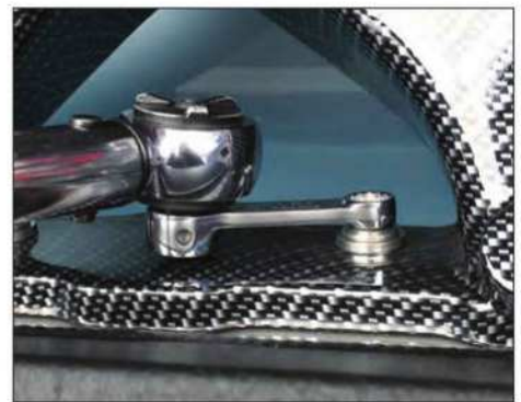
For those situations where you simply don't have access with a socket wrench, a wrench extension makes it easy to apply the desired torque value to an intake manifold bolt, rather than just guessing at bolt tightness.
