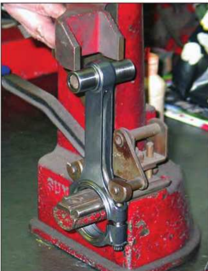
Each connecting rod (especially used) should always be checked for rod deformation, using a rod alignment stand. Here a rod is checked for bend. Note that the upper anvil is resting on top of the wrist pin. With the rod placed onto the tool-centering fixture, use a feeler gauge between the wrist pin surface and the upper checking base.
