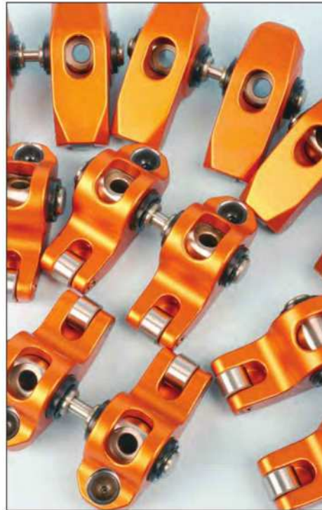
Full-roller rockers made from forged aluminum billets that are CNC machined provide lighter weight and high strength. Pictured here is a set from Harland-Sharp for the GM LS engine.
