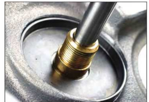
Bronze valve guides can be trimmed to provide needed retainer clearance, providing enough height remains for seal installation.
