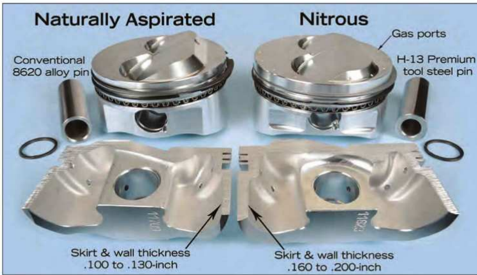
These cutaways provide an example of material thickness in strategic areas between a normally aspirated application (left) and a piston designed for use with heavy nitrous injection. (Photo Courtesy Diamond Racing Products)
