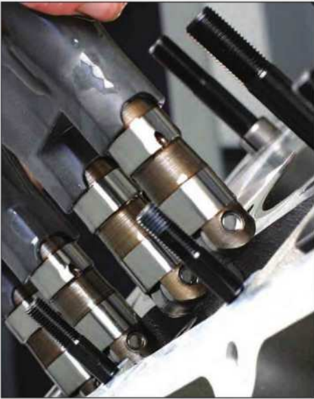
The lifter bucket holds a bank of four roller lifters with the roller tips in plane with the cam.
