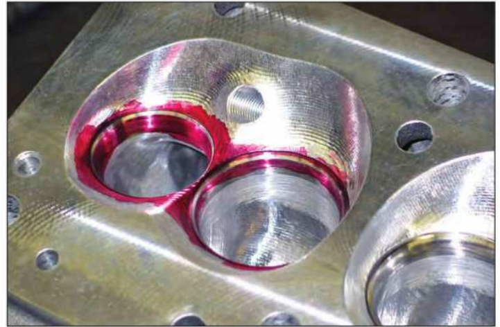
The initial cut is checked for uniformity and concentricity. Note the witness cut through the dye.
