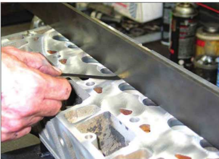
When measuring a cylinder head deck for flatness, use a precision machinists' straightedge and a feeler gauge. Here front-to-rear length is checked.
