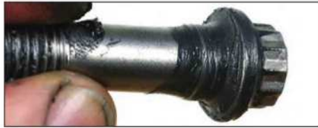
Also apply a coating of assembly lube to the underside of the bolt head. Remember, friction occurs between threads and between the bolt head and the rod cap.
