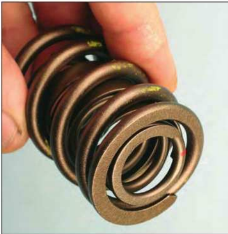
Typical dual-spring with dampener spring. The bottom of the retainer must fit snugly into the ID of the inner spring.
