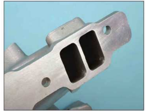
Depending on engine design/type, the manifold may have port pairs that are placed very close together. When port matching, align these divider walls to the heads first, and be careful not to eliminate the gasket sealing area.
