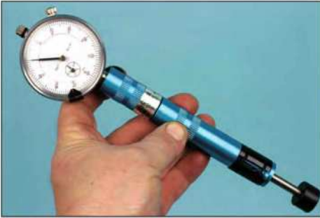
A dial lifter gauge, such as the one made by Foster Tools, allows you to directly read the camshaft lobe.
