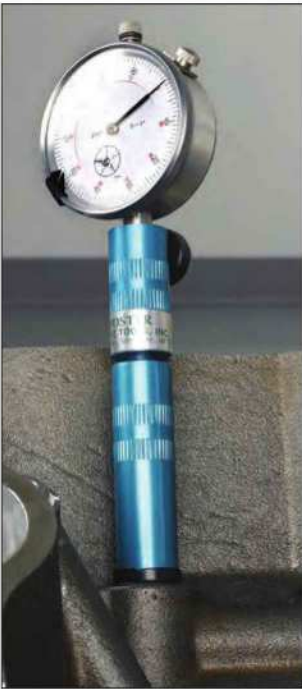
A dial lifter gauge, such as the one made by Foster Tools, allows you to directly read the camshaft lobe.
