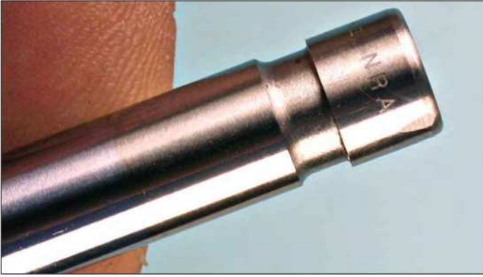
Here's an example of a valve with a traditional square-cut groove. Always inspect the groove style in order to verify the type of locks required. Valve disengagement and failure will result if the wrong style lock is installed.
