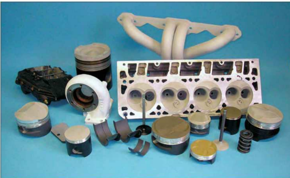
This group of parts helps to illustrate heat barrier and anti-friction coating applications. The examples shown here include high-temperature thermal-barrier coatings on head chambers, piston domes, turbo housing, and headers; anti-friction coatings on skirts, valvestems and bearings; and heat-release (or shedding) coatings on valvesprings. (Photo Courtesy Swain Tech Coatings)
