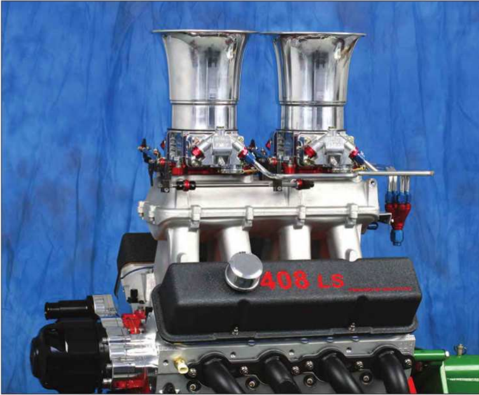
A tunnel ram, or hi-ram, intake manifold such as the Holley Hi-Ram on this custom LS engine features long runners for added volume and air/fuel velocity, benefiting top-end power.
