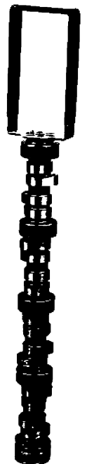
With a handle/grip attached to the cam you greatly reduce the risk of damaging cam bearings.
