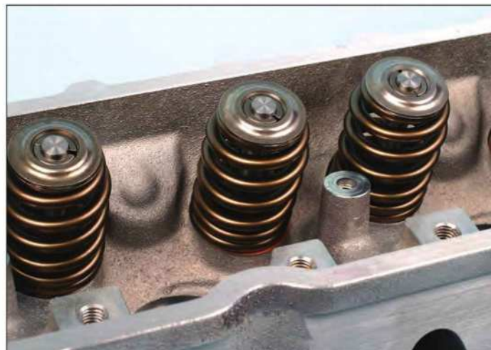
Using steel retainers on beehive springs allows you to save about the same amount of weight as using titanium retainers on full-size non-tapered springs.
