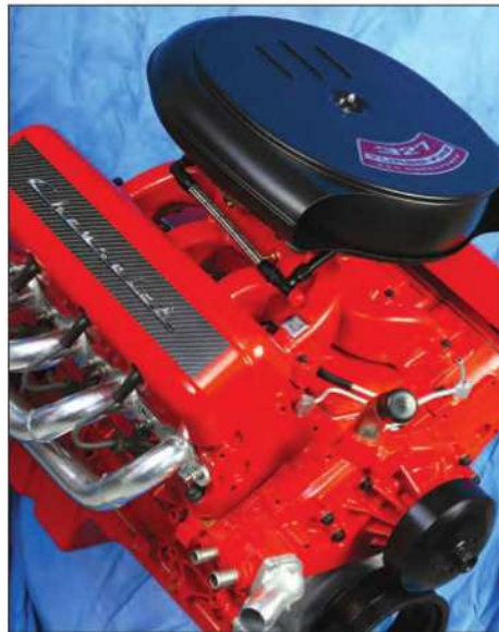
Topped off with a dual-snorkel vintage-style air cleaner, the intake/carb swap from its previous fuel injected format resulted in taking advantage of current-day LS long-block technology while retaining a vintage performance look.
