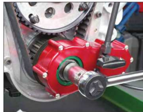
The crank position encoder slips onto the crank snout (using one of their crank-specific keyed aluminum adapters). The encoder is then secured to the block face to prevent encoder body rotation.
