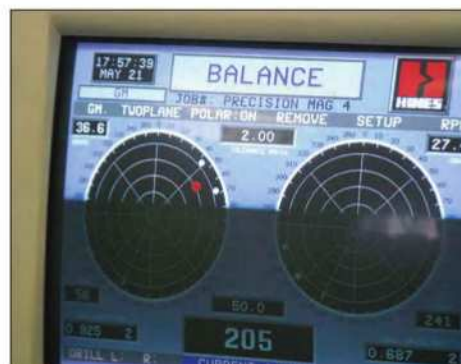
This Hines computer balancer provides a dynamic graph that shows the location required for weight removal or addition, in terms of clock position and depth at the counterweight.
