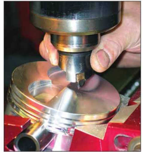
A milling bit adjusted to the proper valve head diameter (with proper clearance added) is used to mill the valve reliefs.
