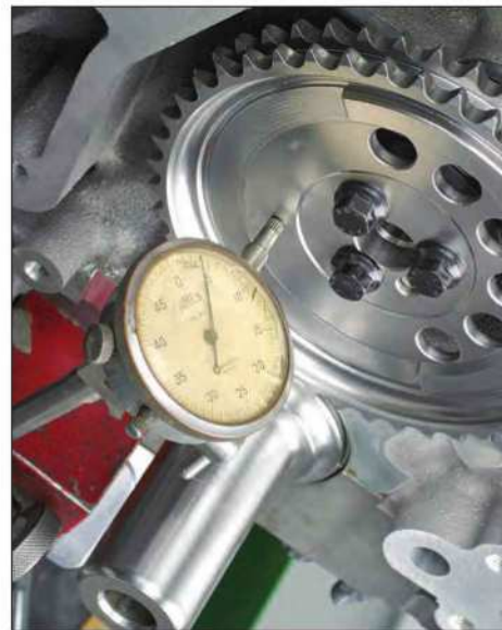
Before attaching the timing chain (or belt), always check camshaft endplay with a dial indicator. Generally, endplay should be somewhere in the range of approximately .003 to .006 inch.
