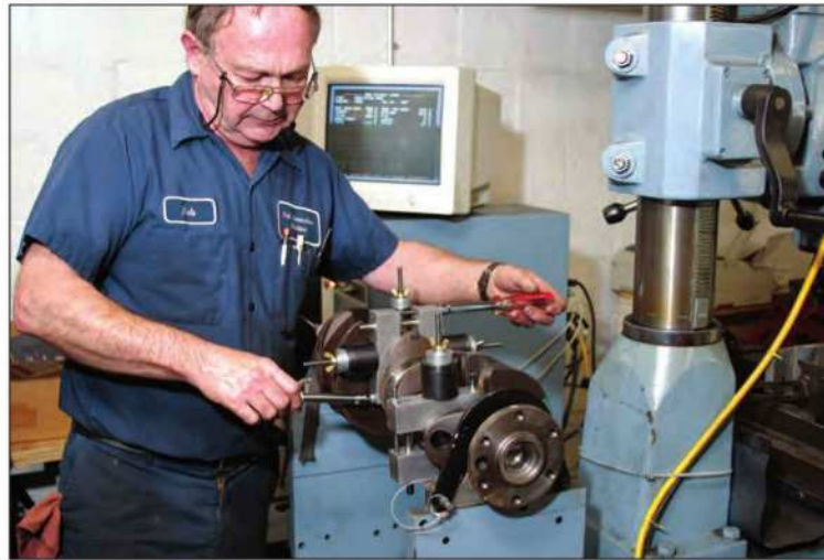
Bobweights should be centered at the width of each rod journal. To save measuring time, machinists often insert an aluminum spacer of a specific thickness to avoid the time required for measuring to center the bobweight.
