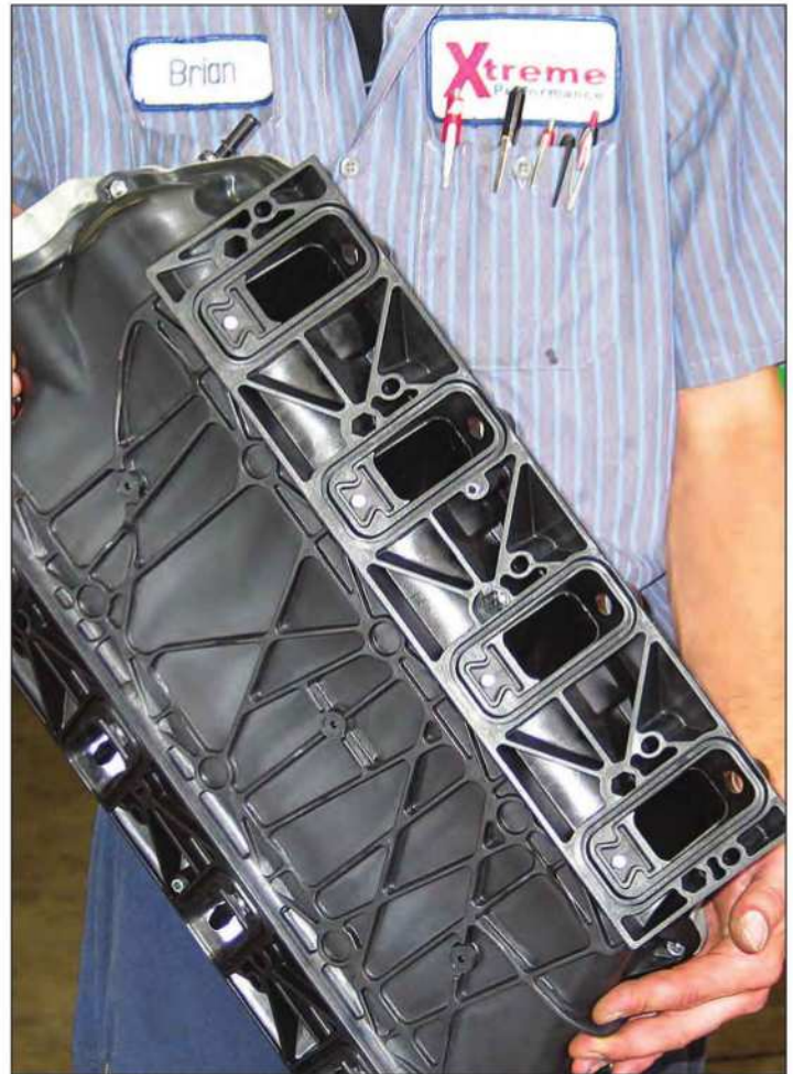
Plastic intake manifolds for fuel-injection setups (OEM or after-market) are basically bolt-ons. Due to the weight-saving designs and preregistered elastomeric-seal grooves, you really can't modify the ports.
