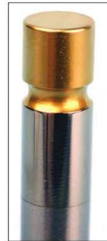
A hard coating applied to the stem tip and lock groove of a titanium valve avoids potential galling where contact exists from a lash cap and the valve lock.
