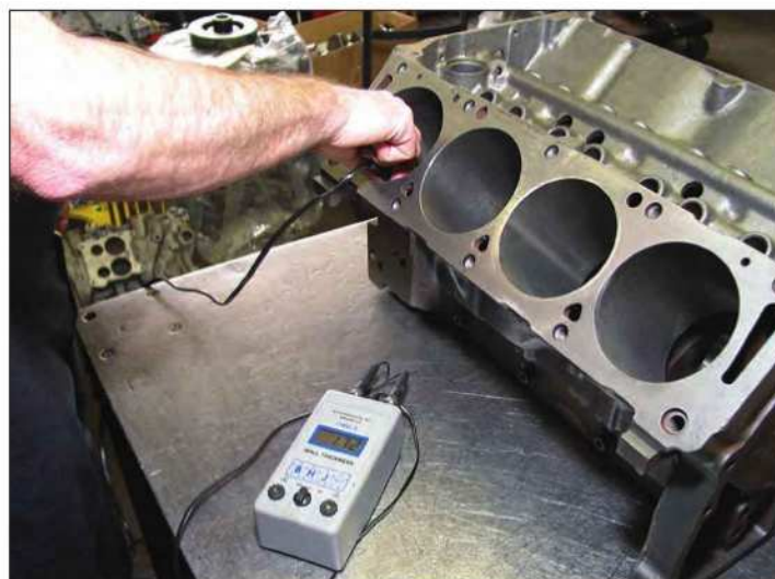
The sensor probe is slowly run along the cylinder wall (in a number of clock positions and from top to bottom) while monitoring the gauge readout.
