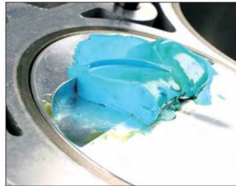
After rotating the crank to run the valves through a complete cycle, remove the head and, using a razor blade, carefully slice a cross section of the clay at the center of the relief. The clay thickness can be measured (carefully) with a dial caliper or small ruler that's incremented in one-thousandths of an inch.
