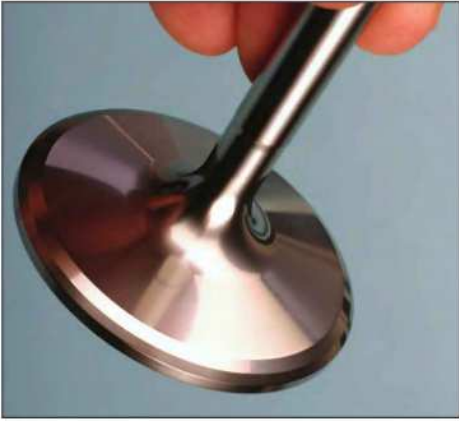
This is an example of a Del West titanium valve that is treated with chromium nitride. This coating offers the additional benefit of allowing valve compatibility with ductile iron or beryllium-copper seats.
