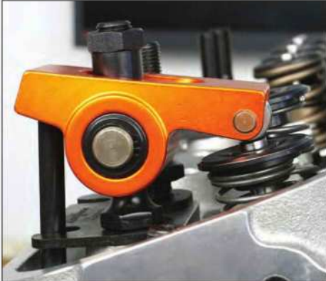
In the midst of the lift cycle, the rocker tip should contact the center of the valve tip.
