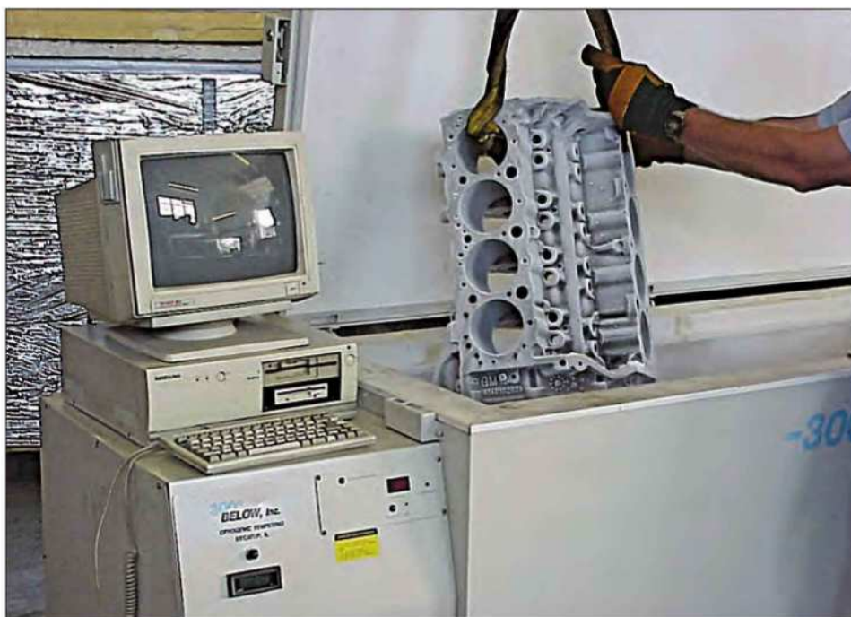
Cryogenic metal tempering requires a specialized, computer-controlled cryo tank that uses liquid nitrogen, in which components are exposed to temperatures at approximately -400 degree F. The pieces are cooled in a slow, controlled manner, then allowed to come back to ambient temperature in a controlled process. The engine block in this photo was removed from the tank only for the photo. Notice the white frosty surface, resulting from the frozen part exposed to room temperature.
