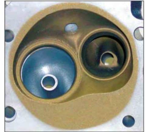
In addition to piston dome coating, the same high-temperature heat-barrier coating may be applied to the combustion chamber, all valve faces, exhaust valve throats, and exhaust valve ports. This completely encapsulates the combustion stream path. (This head was coated by Dart.)
