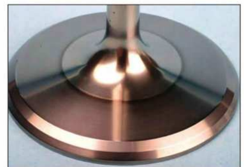
Notice the visible coloration difference at the valve throat. This Del West titanium intake valve has been treated with a chromium nitride (CrN) coating on the valve head and face.
