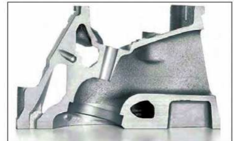
With shallower valve roll angle, the cylinder head can have intake port runners with increased cross section. This is a 6.2-liter LS3 head with 15-degree valve angle. (Photo Courtesy General Motors)
