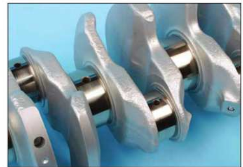
An oil-shedding coating is extremely useful for crankshaft counterweights, allowing oil to more quickly depart from the counterweight surfaces. This reduces the drag that exists because of clinging oil, which in turn reduces parasitic power loss.
