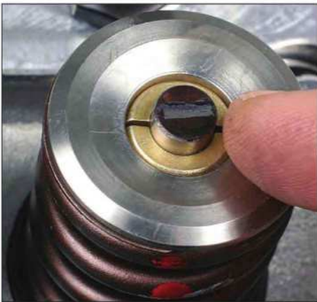
In the midst of the lift cycle, the rocker tip should contact the center of the valve tip.
