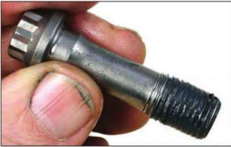
When applying assembly lube to the rod bolts, apply an even coating to the bolt threads.
