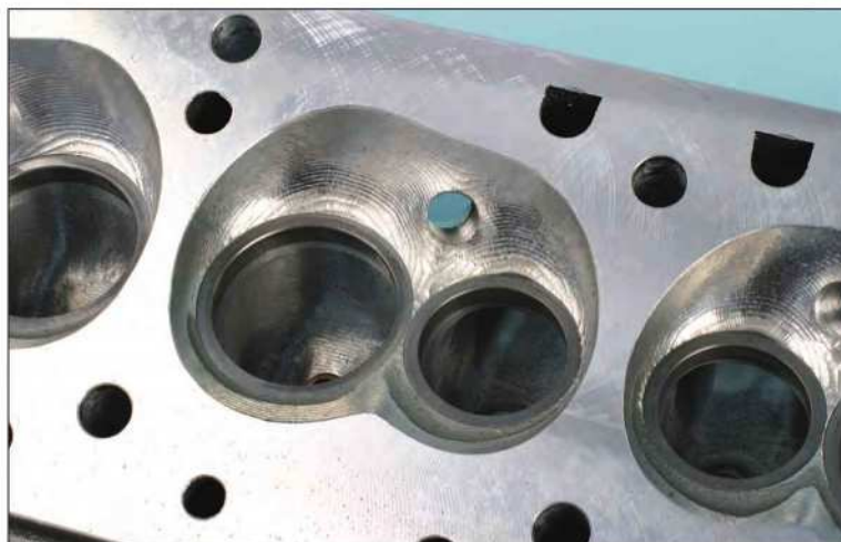
Bare cylinder heads usually have raw, unfinished valve seats that allow the machinist to create the desired valve depth.
