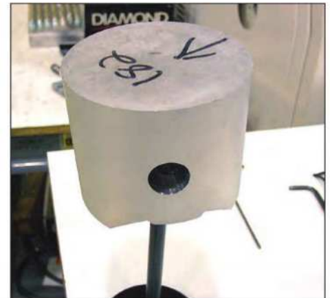
Custom forged pistons start off as billet blanks, followed by placement of the pin bore. (Photo Courtesy Diamond Racing Products)
