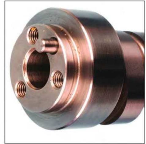
Flat-tappet cams have lobes that are slightly tapered, to force the flat-tappet lifters to rotate. This lobe taper also causes the cam to walk fore/aft slightly. Since a roller cam doesn't need (and can't use) this taper, a roller cam needs a method to prevent this walk. Many roller cams have a stepped nose, designed to be stopped from walking forward by a retainer plate. Otherwise, a cam button is needed; this drops into the center of the cam nose and takes up the space between the cam nose and the rear of the timing cover.
