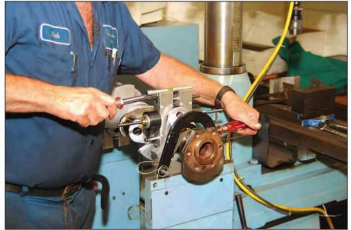
Each bobweight is placed with the weight side 90 degrees to each rod journal.
