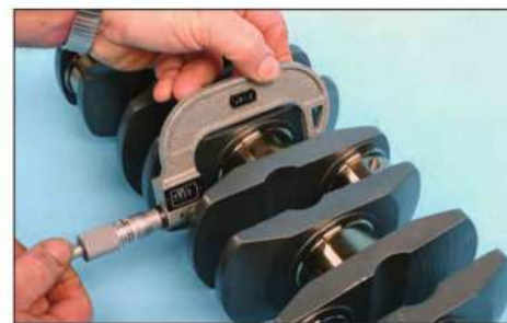
When measuring crank journals, be careful to avoid contacting the micrometer's anvils to the journal's oil feed hole.
