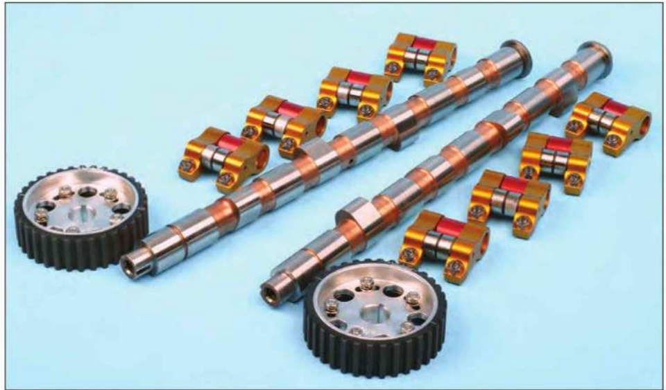
OHC setups use cam followers that directly transmit valve action from the cam lobes.
