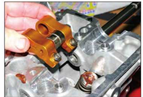
This Ferrea aluminum full-roller cam follower is being fitted to a Honda race head. The large needle-bearing roller rides under the cam lobe, and the adjusters ride directly on the valves. A follower pivot shaft is inserted through the head to provide a pivot point.
