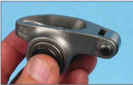
A full-roller rocker has a needle-bearing trunnion for the pivot point and a roller bearing for valve tip contact.
