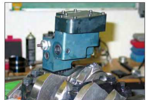
The big advantage of the billet pumps is the elimination of a separate pickup, so pickup tube damage such as loosening or cracking due to engine vibration is eliminated.
