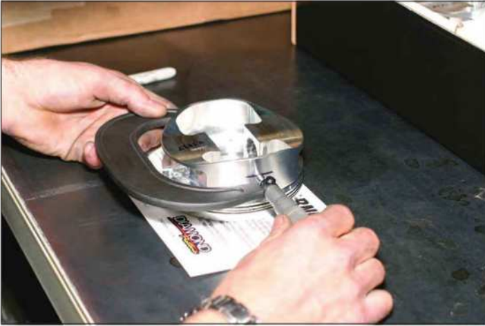
Never assume anything. Whether you plan to use OEM or after-market pistons, always measure each piston skirt diameter at the skirt height location specified by the piston manufacturer, for your final cylinder diameter, including desired piston-to-wall clearance. Final cylinder diameter is always based on the actual piston-skirt diameter.
