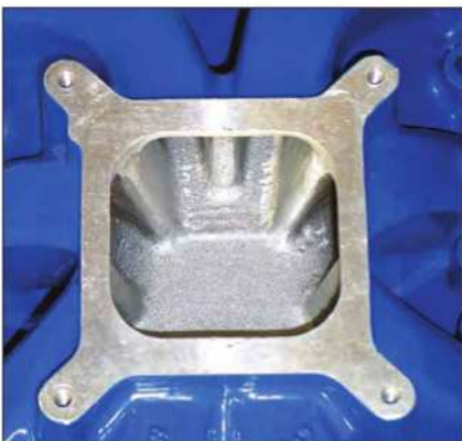
The popular F.A.S.T. composite intake manifold for fuel-injected applications consists of a lower section (runners) and a top section that incorporates the throttle body inlet. Shown here is a unit for late-model Corvette.
