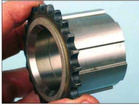
The pump's driven gear slips over and engages the drive gear, which installs onto the crankshaft snout. This OEM-LS drive gear has an integrated timing chain gear.
