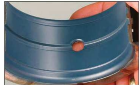
MAHLE Clevite, for example, uses a polymer-based moly-graphite coating on its performance bearings.
