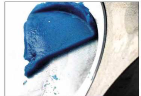
Clay is also good for checking the angle of valve attack relative to the angle of the piston's valve pocket.
