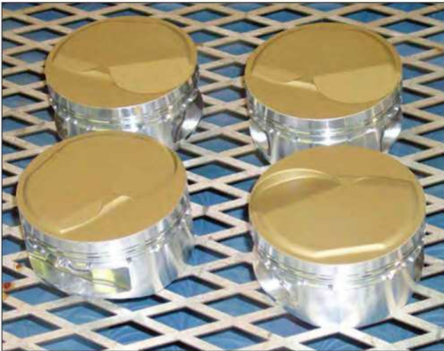
The set of pistons in this shot have had only the domes treated to a ceramic thermal barrier coating.
