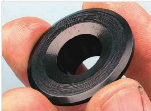
This is a bead-lock valve lock. Remember, this style is only to be used with a bead-lock valve.
