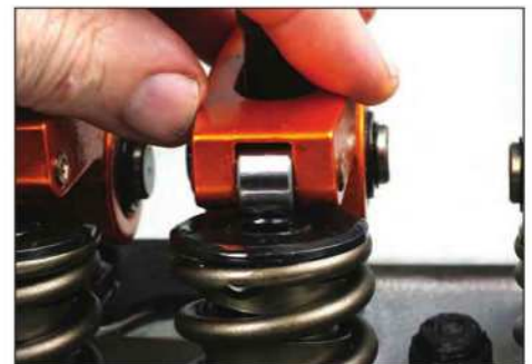
During test fitting, verify that the rocker tip is centered to the valvestem tip. If you're using pushrod guideplates, the guideplates may require adjustment for positioning.
