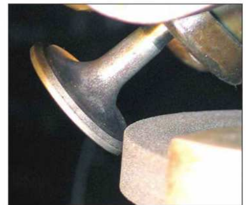
Valves can be refaced (on a collet machine or a centerless grinding machine). Remember that regrinding the sealing face of the valve sinks the valve farther into the seat, increasing chamber volume and decreasing compression ratio.
