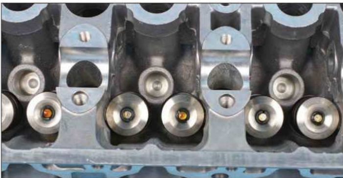
Special spring compressors are required when removing/installing valves and springs on many OHC cylinder heads because of the tight confines.
