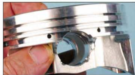
Piston compression distance (also called compression height) is measured from the centerline of the wrist pin bore to the flat (or quench) surface of the piston top. This does not include any protruding dome.
