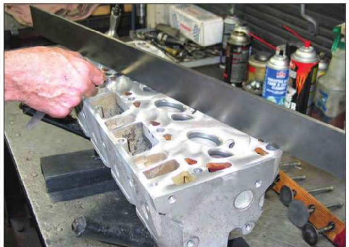
Also measure the head deck diagonally from corner to corner, at all four corners. Generally speaking, maximum allowable deviation is about .002 inch.
