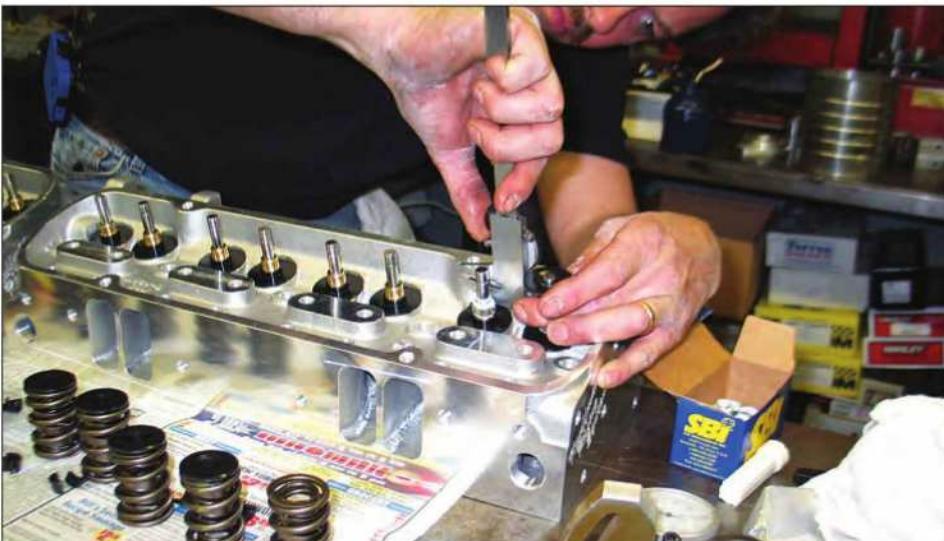
Once initial cuts have been made, valves are installed to check for valve depth. The goal is to establish equal depth of all valves.
