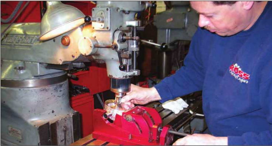
A dedicated precision piston vise allows the piston to be secured in the correct valve angle prior to pocket milling.
