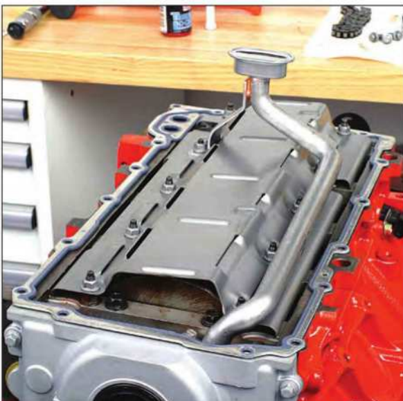
If the pump is located far from the sump, the tube will be long and require at least one additional support bracket to support the weight and length of the pickup tube. It is usually fastened to a main cap bolt or stud. Here is a stock type pickup on a GM LS engine. The sheet-metal tray seen here serves as a windage tray, which protects the crankshaft from oil splashback from the pan. This reduces parasitic oil drag on the crank counterweights and rod big ends.
