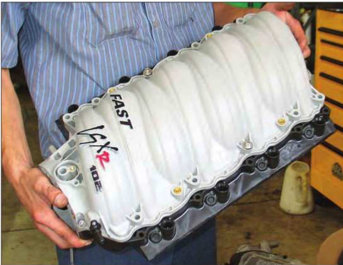
The popular F.A.S.T. composite intake manifold for fuel-injected applications consists of a lower section (runners) and a top section that incorporates the throttle body inlet. Shown here is a unit for late-model Corvette.
