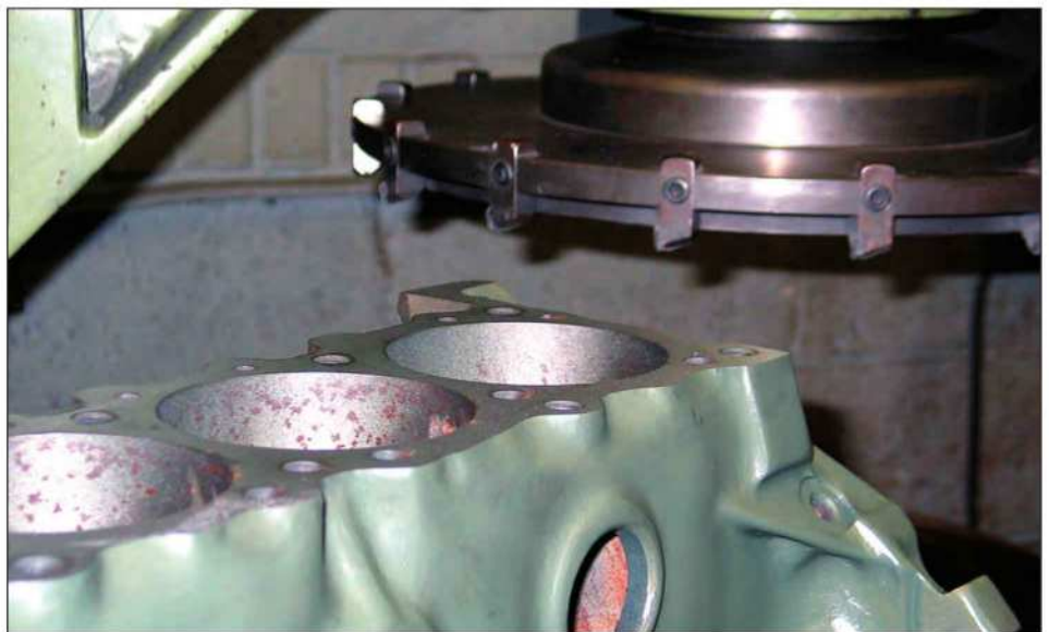
Resurfacing is best done with milling bits to achieve the desired surface finish.
