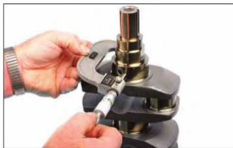
Measure journal diameters in several locations (different clock positions), and perform a backup measurement with a different micrometer.
