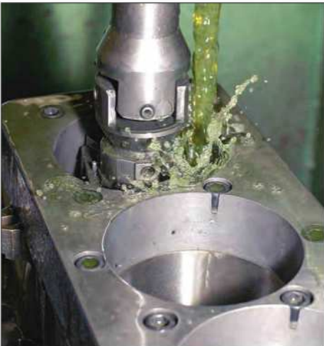
Honing coolant is constantly supplied as the honing stones rotate and travel through the cylinder, keeping the stones clean and reducing heat buildup.
