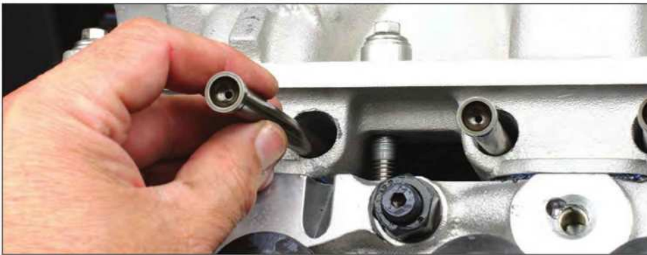
The vintage Ford FE big-block manifolds have pushrod holes. For high-performance applications where larger diameter pushrods and/or high-lift cams are used, these holes may require slight enlargement or elongation. This must be checked during test fitting, with an assembled short block, heads, and rockers installed.
