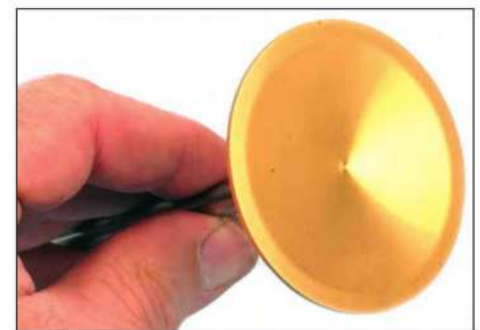
A specialized titanium nitride coating on the valve face provides superior protection from heat and carbon deposit buildup.
