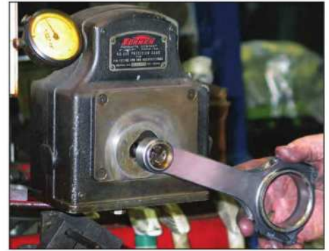
The same rod bore gauge is used to check the rod's pin bore. If using aftermarket performance full-floating rods, diameter is based on recommended oil clearance to the wrist pins.
