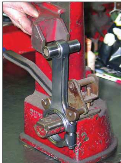
The same fixture is used to inspect the rod for twist, with the upper anvil contacting the side of the rod pin. Any measured bend or twist beyond .003 inch is cause for concern.
