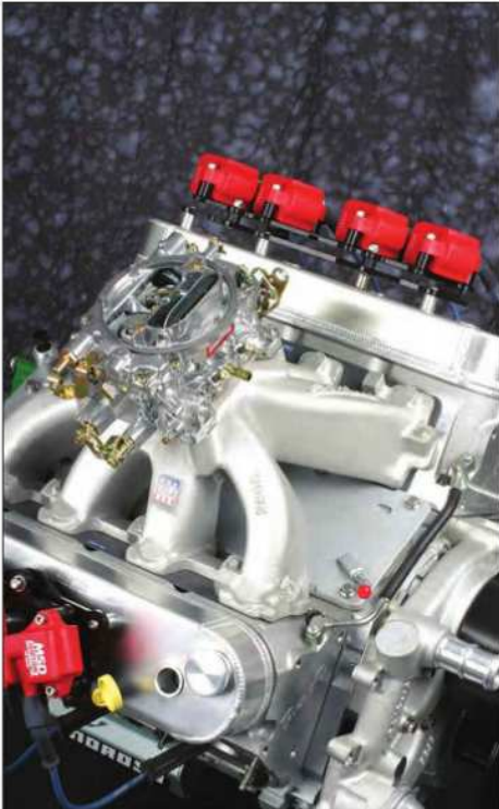
Converting a GM LS engine to old-school carburetion is embarrassingly simple, requiring only a manifold, carb, and an MSD ignition controller. No ECM required.
