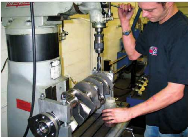
When weight must be removed from a crank counterweight, it is done on an overhead drill press. Some balancing machines incorporate a drill while a separate drill press is required for other systems.
