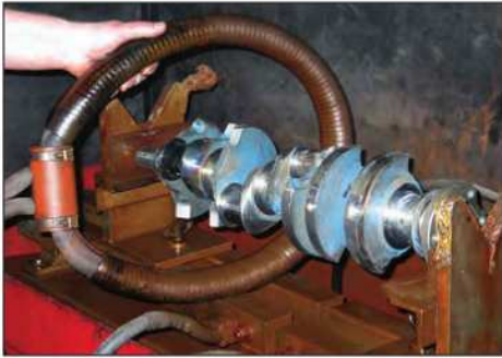
A magnetic particle inspection station (a wet bench) has a large-diameter magnet that creates a magnetic field. The component being checked passes through this field.
