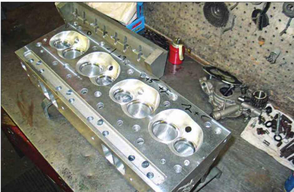
This Pontiac big-block head has been checked for initial valve depth. Note the depth markings adjacent to each chamber. In this example, initial depths ranged from -0.001 to +0.005 inch.
