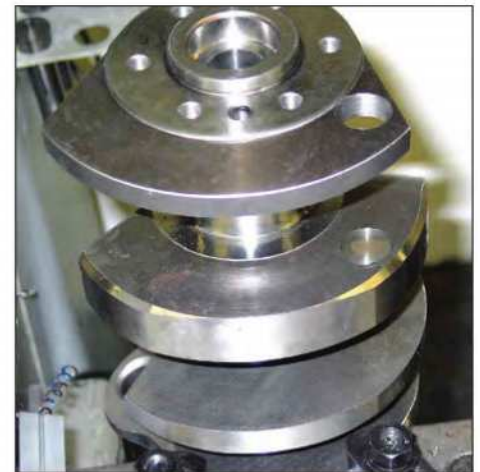
When weight must be removed from a crank counterweight, it is done on an overhead drill press. Some balancing machines incorporate a drill while a separate drill press is required for other systems.
