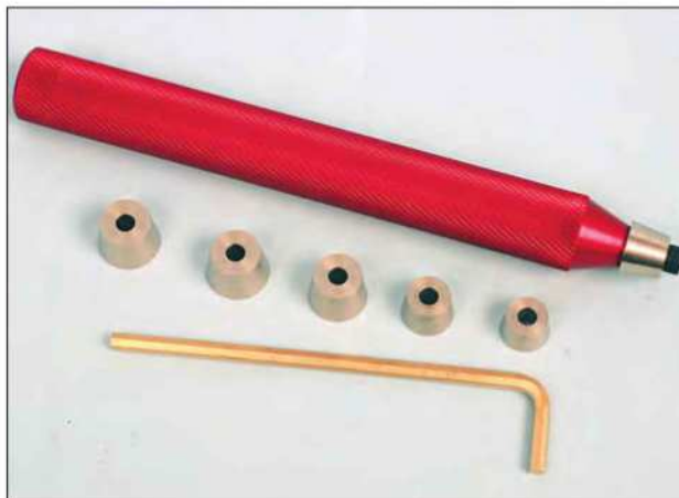
Hardened steel lash caps are designed to protect the relatively soft tip of a titanium valve although titanium valves are now available with built-in hard tips. Lash caps are also useful in fine-tuning rocker arm geometry and valve lash range and are available in various thicknesses. The lash cap should fit snugly onto the valve tip.
