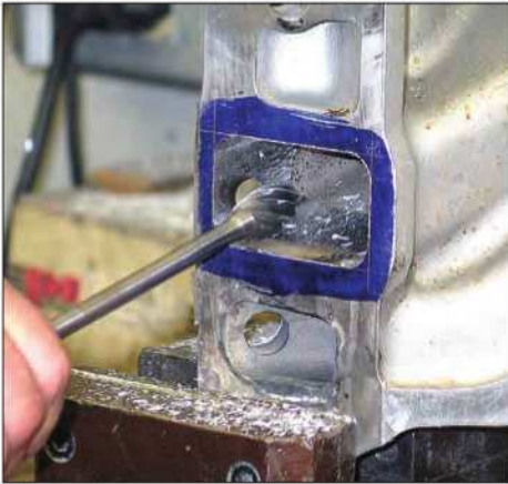
After removing material around the port edges to your scribe lines, taper blend the cut inside the runner at a depth of about 1 inch.
