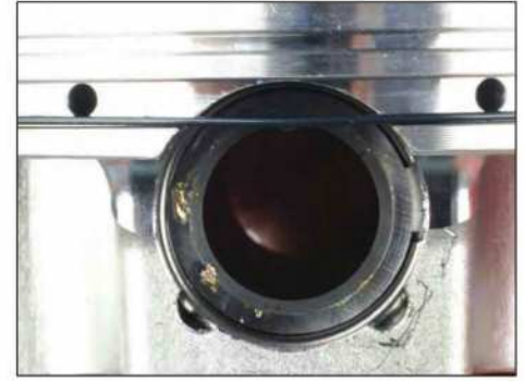
This is an example of an oil ring support rail installed to the floor of the oil ring groove. The rod and piston pin must be installed before installing the rings, due to the wrist pin being captive behind the support rail.
