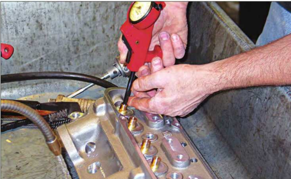
During guide honing, the gauge is used to check/verify guide ID through the entire length of the guide.
