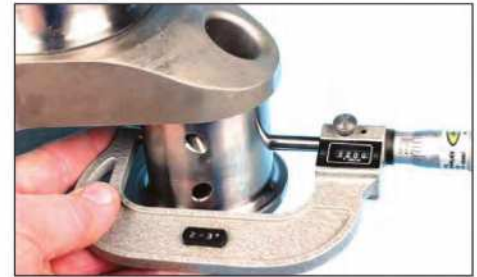
Use a quality calibrated micrometer to measure main and rod journal diameters. Avoid cheap gauges, as accuracy is critical. Also, check your mic for calibration before each use, using the calibration checking standards (these should be included in a quality micrometer kit).
