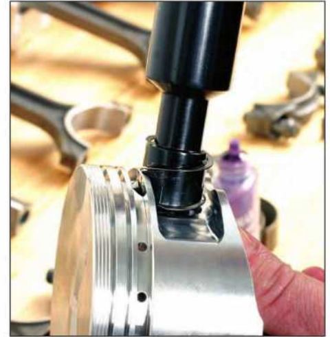
Specialty installation tools for spiral locks are easy to use. Spread the spiral, thread it onto the tool, enter the tool at a slight angle, and rotate counterclockwise. Straighten the tool out (parallel to the pin) and continue to rotate the tool counterclockwise until the lock snaps into the groove. These tools are available for both spiral locks and wire locks, in a variety of diameter sizes to match the pin bore size. Steel versions run about $75 each and plastic versions are about $25 (made by Lock-In-Tool).
