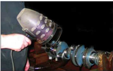
Once the component has been lightly magnetized, a dye fluid is applied and inspection is done using a UV light (or black light). These machines usually have a curtain surrounding the testing area for better UV viewing. Here Bob Fall, of Fall Automotive Machine in Toledo, Ohio, prepares to inspect a crankshaft. The curtain is left open only for the sake of this photo.
