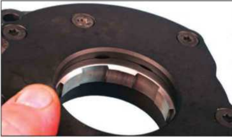
Crank-driven oil pumps have a driven gear that have a series of broad teeth.
