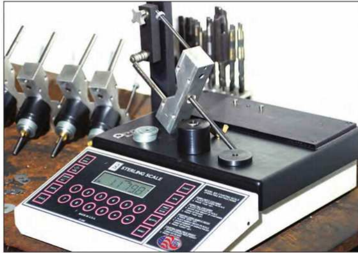
During makeup of the bobweights, they're weighed on the digital scale and adjusted (with more or fewer weights to match the required weight).
