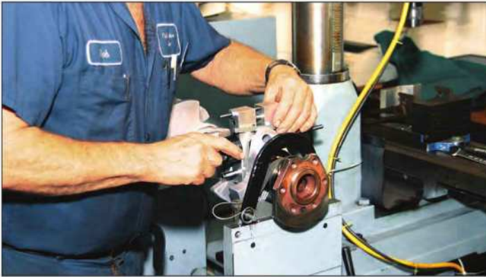
Bobweights should be centered at the width of each rod journal. To save measuring time, machinists often insert an aluminum spacer of a specific thickness to avoid the time required for measuring to center the bobweight.
