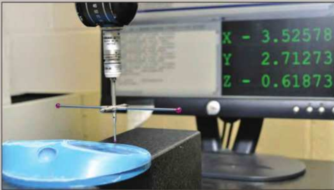
During CMM processing, a digital probe travels across the entire combustion chamber model, providing all dome information to the system database. (Photo Courtesy Diamond Racing Products)
