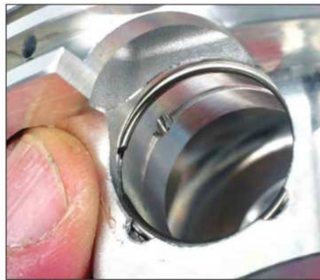
Here's a wire lock fully installed. Be sure to position a wire lock with the lock gap away from the small access notches. During future removal, you'll be able to insert a pick through one of the notches to grab the lock.
