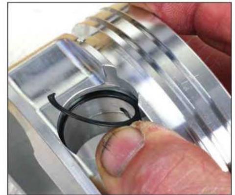
Spiral locks can be tricky at first, but once you install a few it becomes second nature. After gently spreading the spiral apart, insert one end and "walk" the remainder in a counterclockwise direction into the groove until the final end snaps into place. Some installers use their fingers along with a small, flat-blade screwdriver, but specialty installer tools are available.
