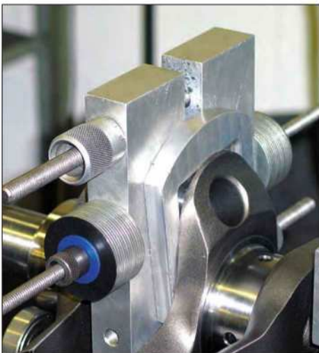
Shown here is a spacer inserted on one side of a bobweight. With the bobweight pushed up against the spacer, the bobweight's halves are secured together, and then the spacer is removed.
