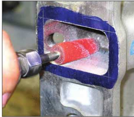
Blend into the port to fully smooth out the surface, again, at about a 1-inch depth. If you prefer a smoother surface (more of a polish), then go over the surfaces with 80-grit.
