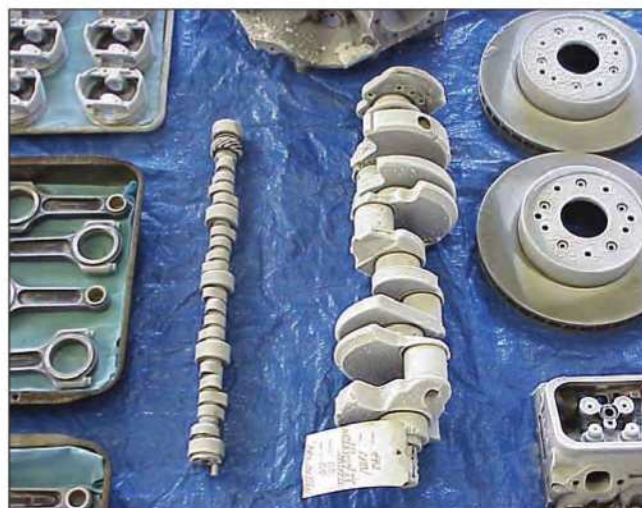
A wide range of components can benefit from cryogenic tempering, including blocks, heads, rods, cranks, cams, rockers, and brake rotors. (Photo Courtesy 300 Below)
