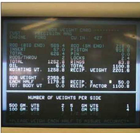
The monitor on this balancer's screen displays all of the weight data input by the technician.
