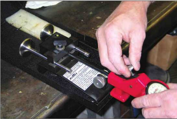
Prior to honing new valve guides, the guide ID gauge is adjusted for valve stem diameter plus specified oil clearance.
